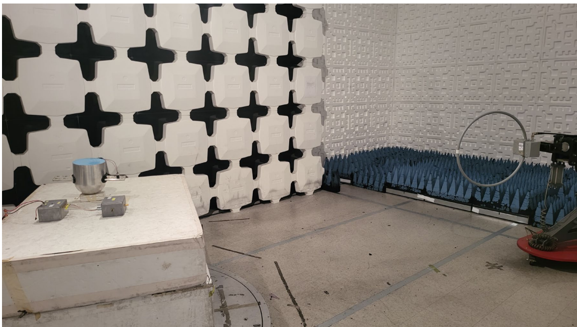
Figure 2. Radiated Emissions Test Setup, .15 MHz to 30 MHz
