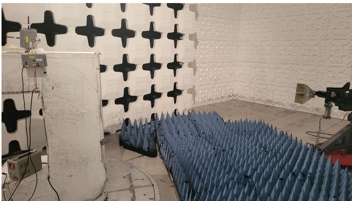
Figure 5. Radiated Emission Test Setup, above 1 GHz
