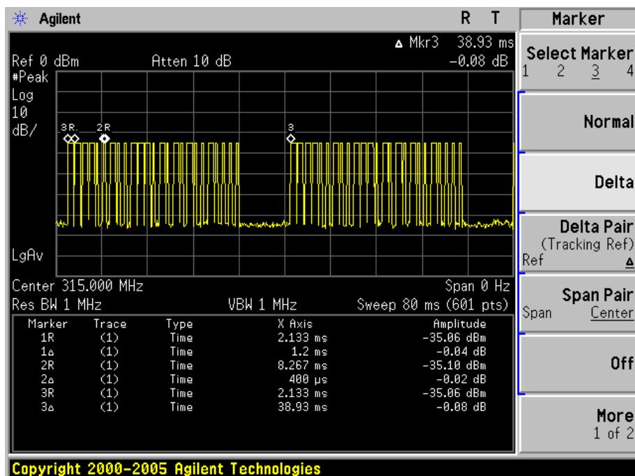
$$\text{DCCF} = -20 \log[(1.2 \text{ms} \times 12 + 0.4 \text{ms} \times 13)] / 38.93 \text{ms} = -20 \log(19.6 / 38.93) = 5.96 \text{dB}$$
