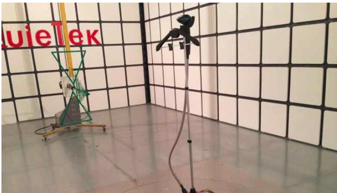
Description: Radiated Emission Test Setup for 1~18GHz
