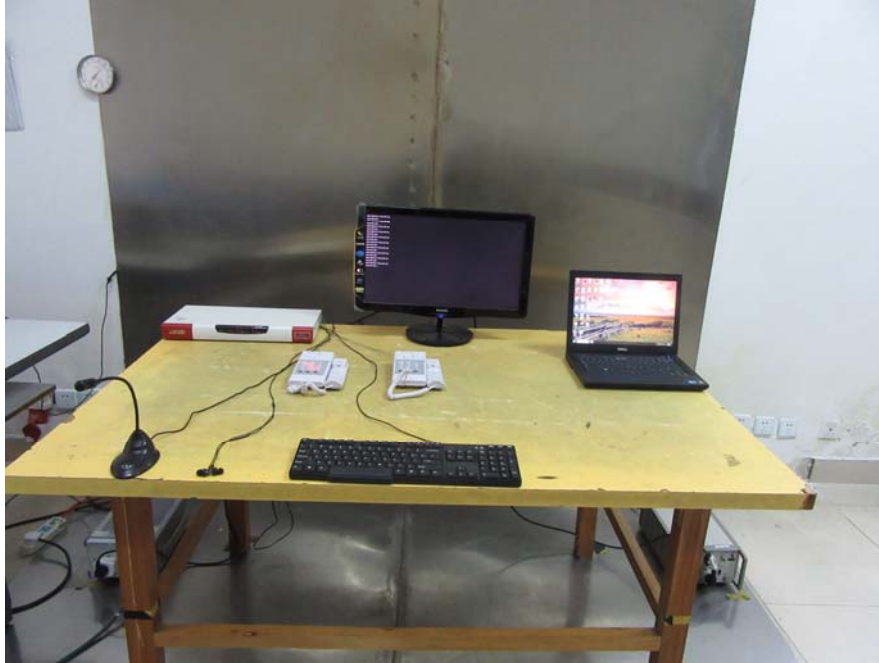
Conducted Emissions Test Setup – Front View
