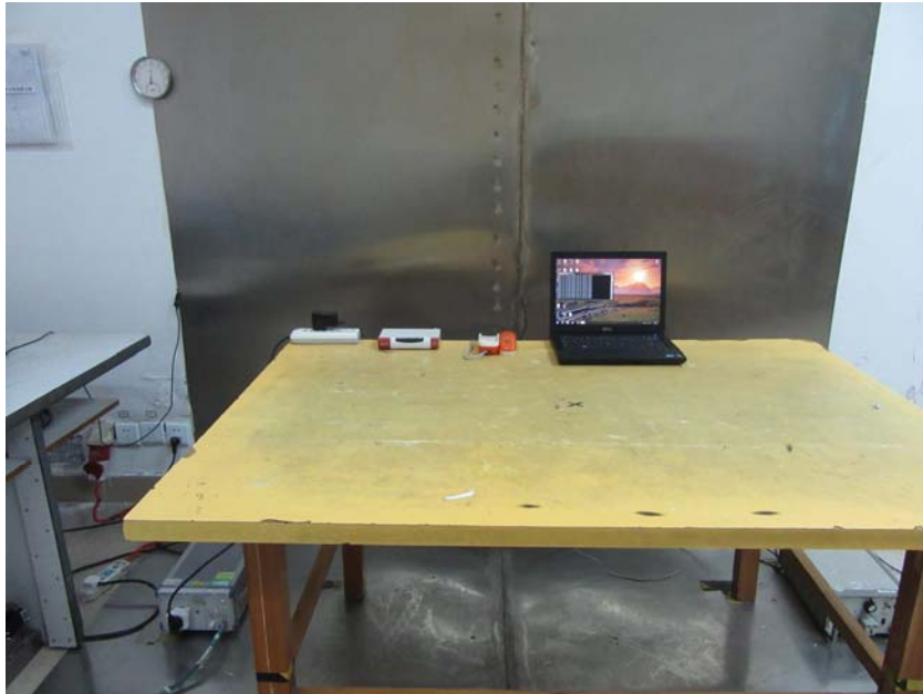
Conducted Emissions Test Setup – Front View
