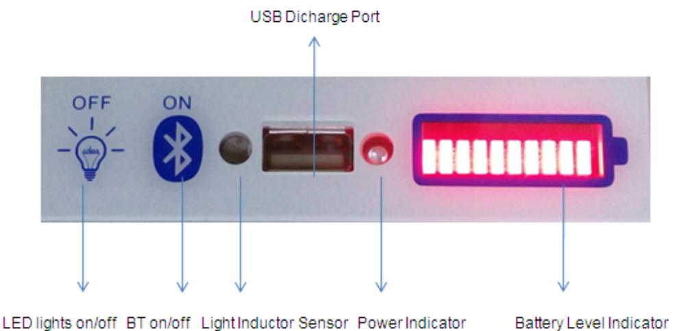
3.8.1: Battery Level Indicator: 10 bar LED lights to show battery level, more accurate
