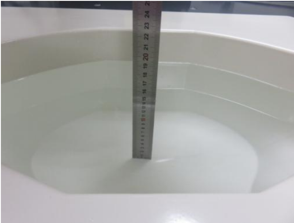
Photograph of the depth in the Body Phantom (2600MHz, 15.2cm depth)
