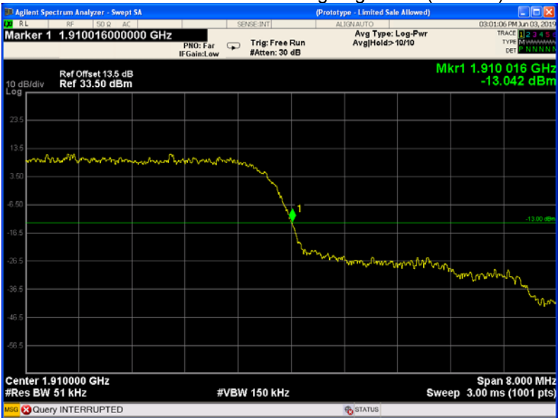
WCDMA band II band edge-right side (HSUPA)
