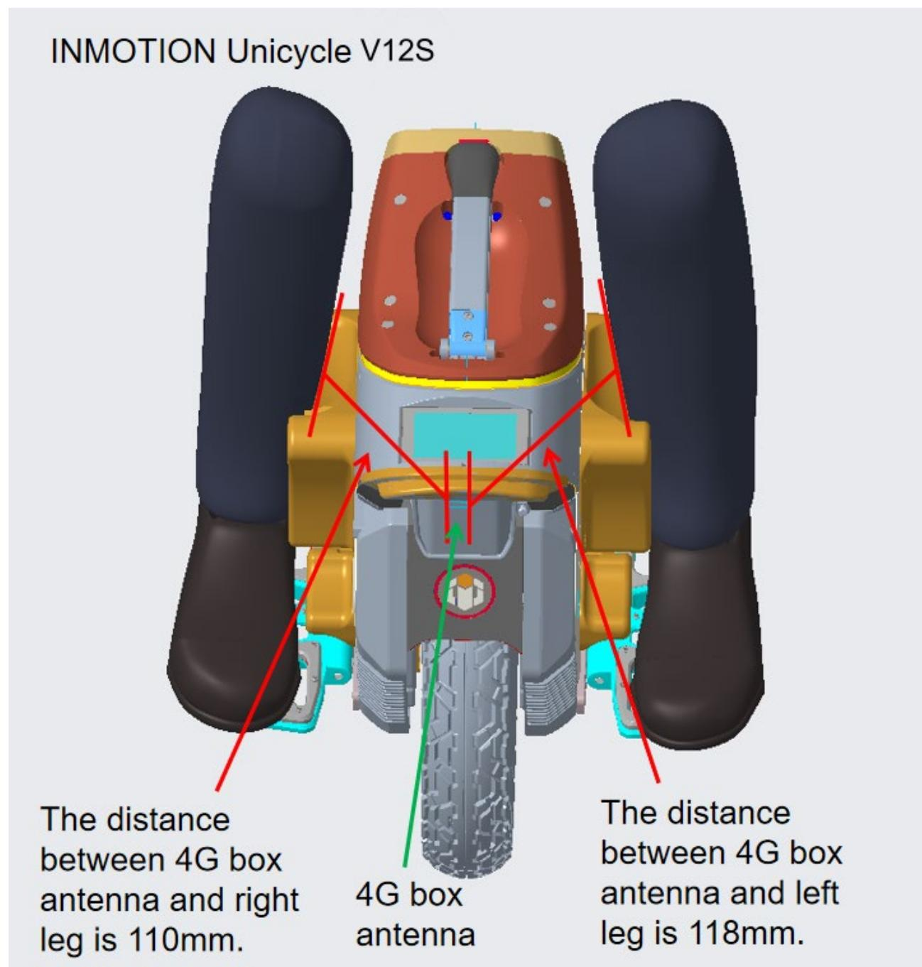
b) Calculate the Min. SAR Test Exclusion Threshold (mW) at a distance of 110mm.
