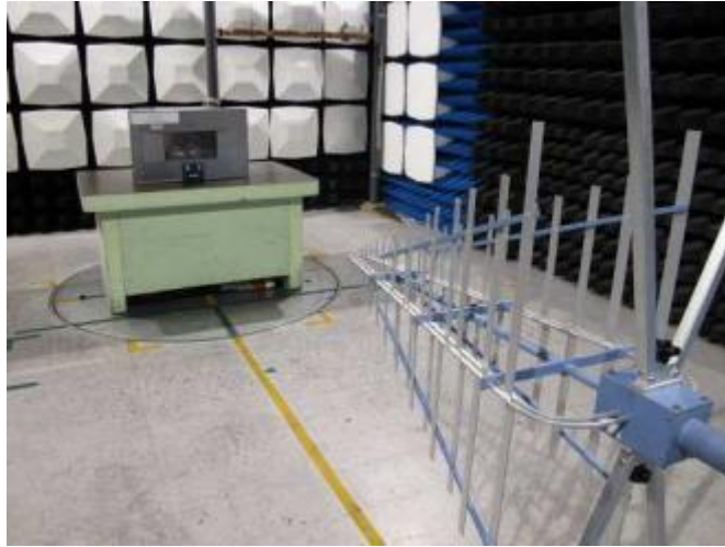
Photo of the EUT during Radiated emission test 30 MHz – 1000 MHz
