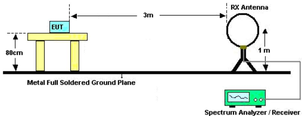
For radiated emissions from 30MHz to 1GHz
