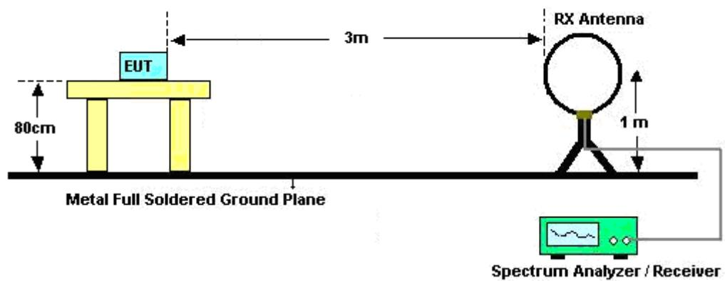
For radiated emissions from 30MHz to 1GHz
