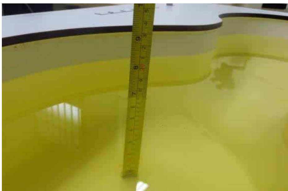
Liquid depth in the Flat Phantom (1900 MHz) (depth>15cm)
