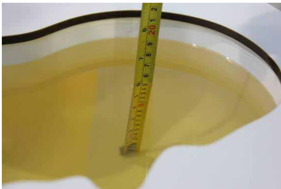
Liquid depth in the Head Phantom (900 MHz) (depth>15cm)
