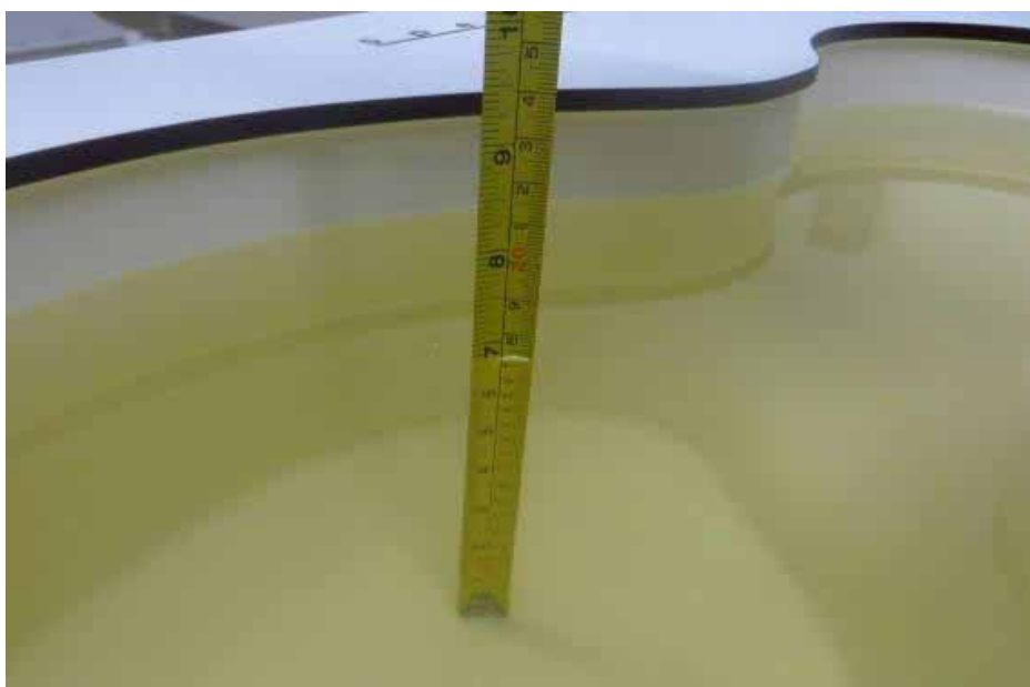
Liquid depth in the Body Phantom (2450 MHz) (depth>15cm)
