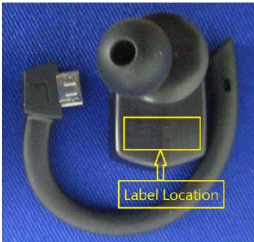
The label shown shall be permanently affixed at a conspicuous location on the device and be readily visible to the user at the time of purchase (Labeling requirements per 2.925)
