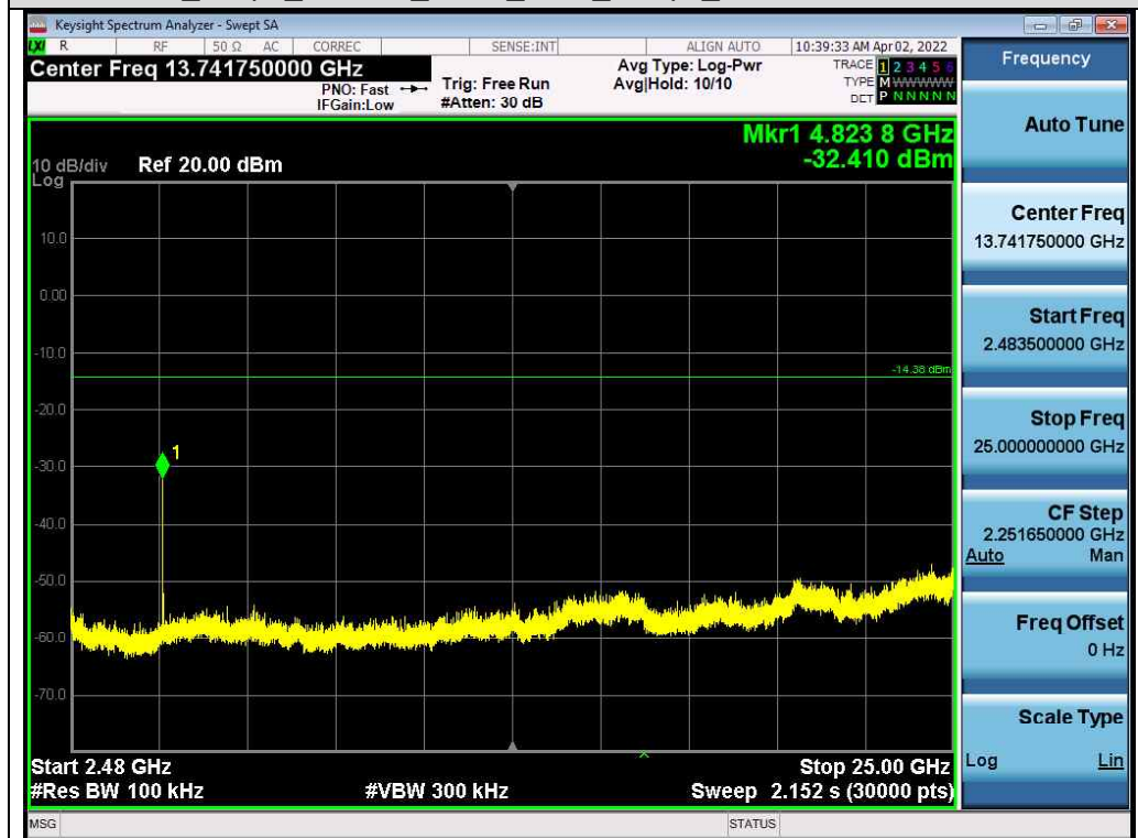
Test_Graph_802.11b_ANT1_2412_1Mbps_Higher Band Emissions
