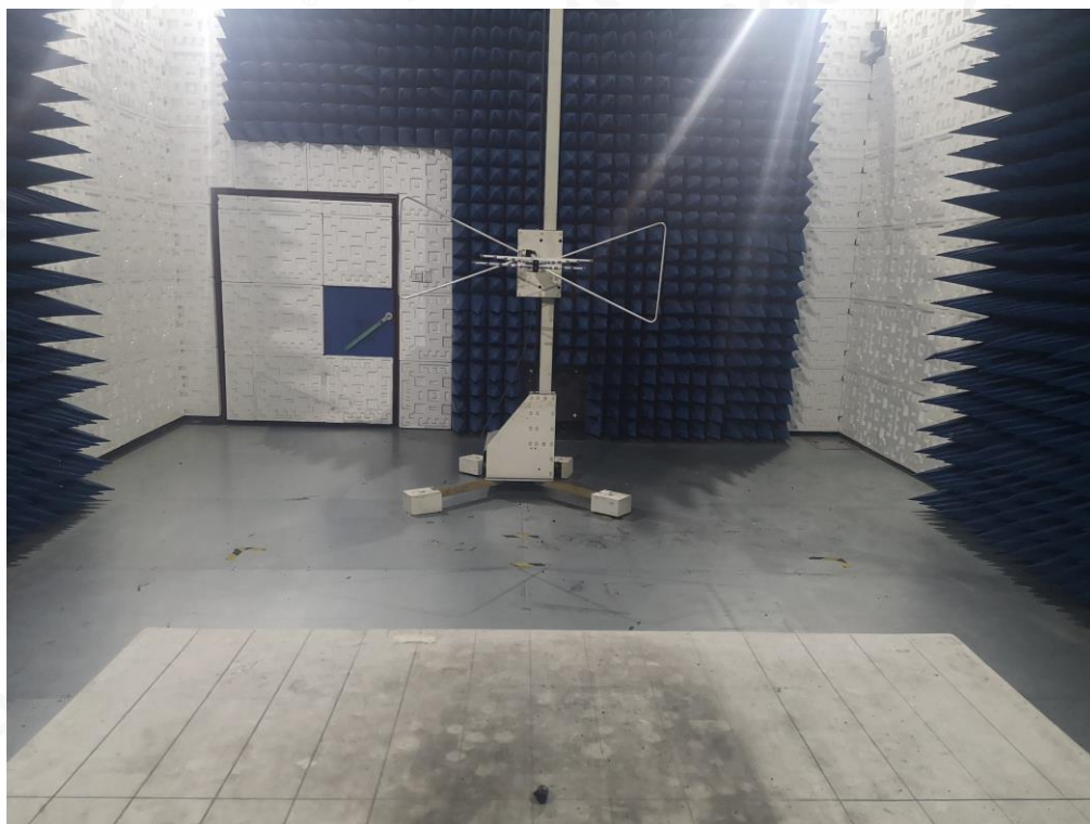
RADIATED EMISSION TEST SETUP ABOVE 1GHZ
