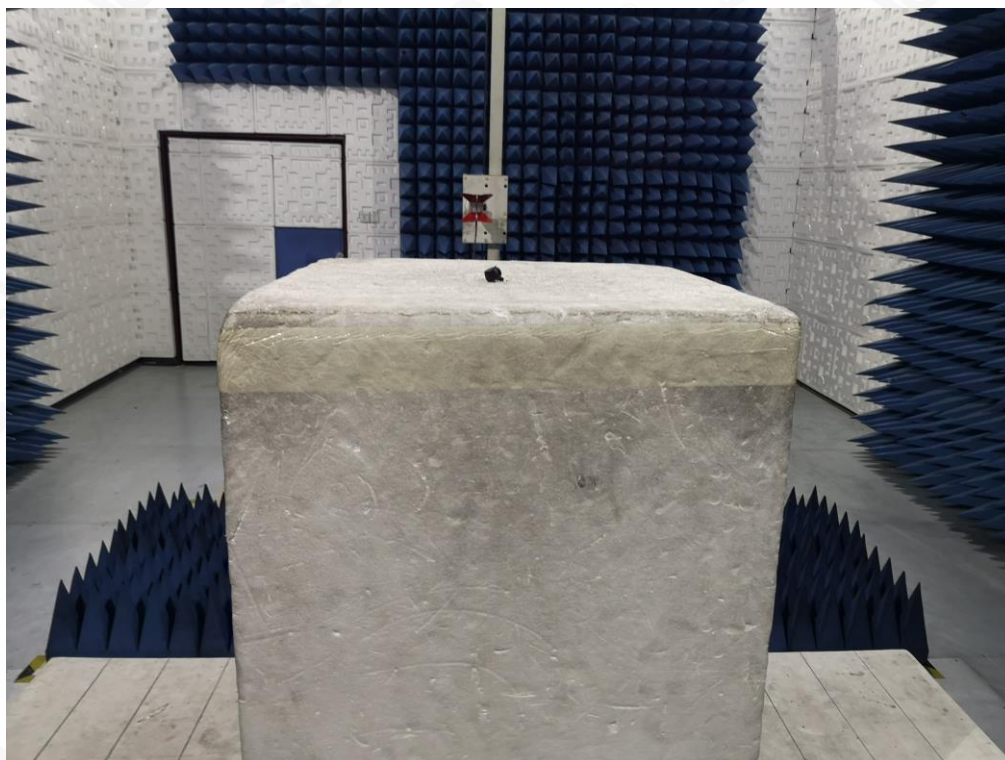
RADIATED EMISSION TEST SETUP ABOVE 1GHZ
