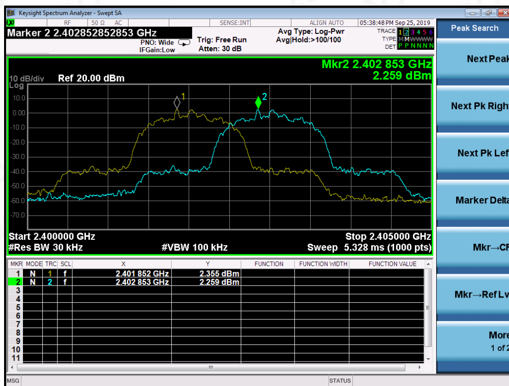
TEST PLOT FOR FREQUENCY SEPARATION
