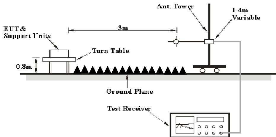
The radiated emission Below 1GHz tests were performed in the 3 meters chamber test site, above 1GHz tests were performed in the 3 meters chamber test site, using the setup accordance with the ANSI C63.4-2014. The specification used was the FCC Part 15.109 Class B limits.
