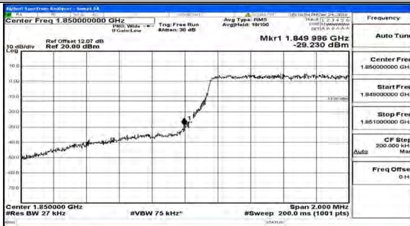
Band Edge Test Graph(s) (Channel Bandwidth: 1.4 MHz)_LCH_16QAM
