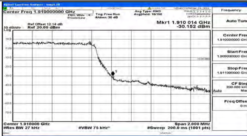
Band Edge Test Graph(s) (Channel Bandwidth: 1.4 MHz)_HCH_QPSK
