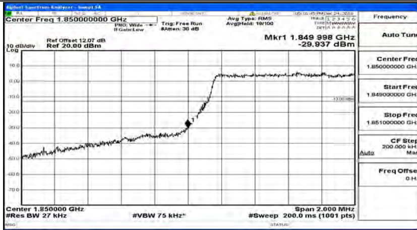
Band Edge Test Graph(s) (Channel Bandwidth: 1.4 MHz)_LCH_QPSK
