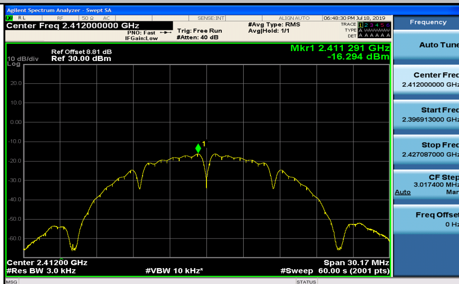
Maximum(average) power spectral density_11B_2437_Ant1
