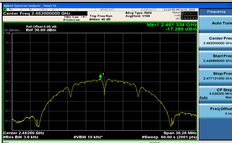
Maximum(average) power spectral density_11B_2462_Ant2
