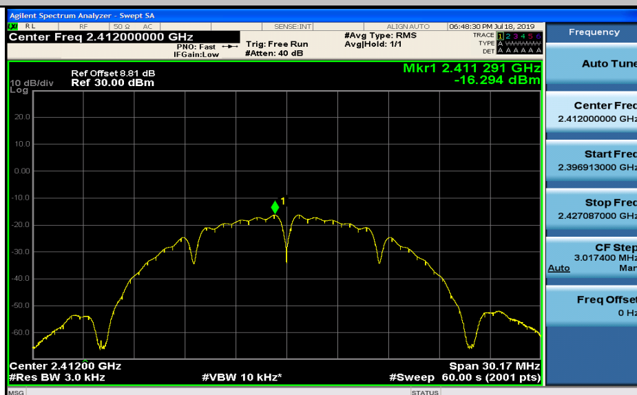
Maximum(average) power spectral density_11B_2462_Ant1
