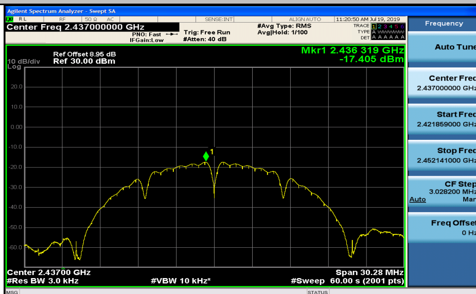
Maximum(average) power spectral density_11B_2462_Ant2
