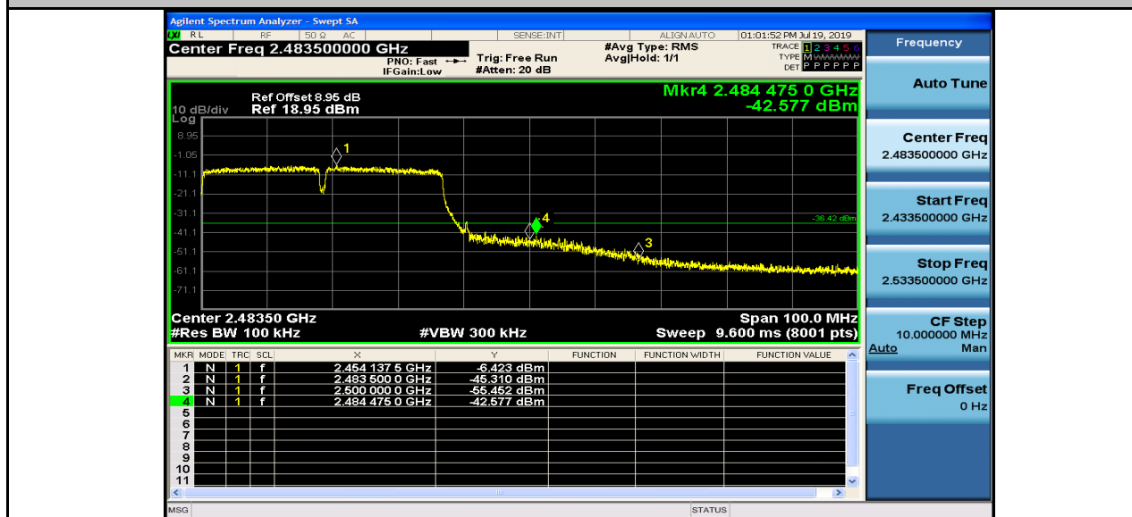
Band-edge for RF Conducted Emissions_11N40SISO_2452_Ant2
