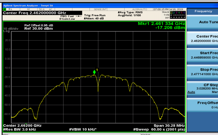
Maximum(average) power spectral density_11B_2462_Ant1
