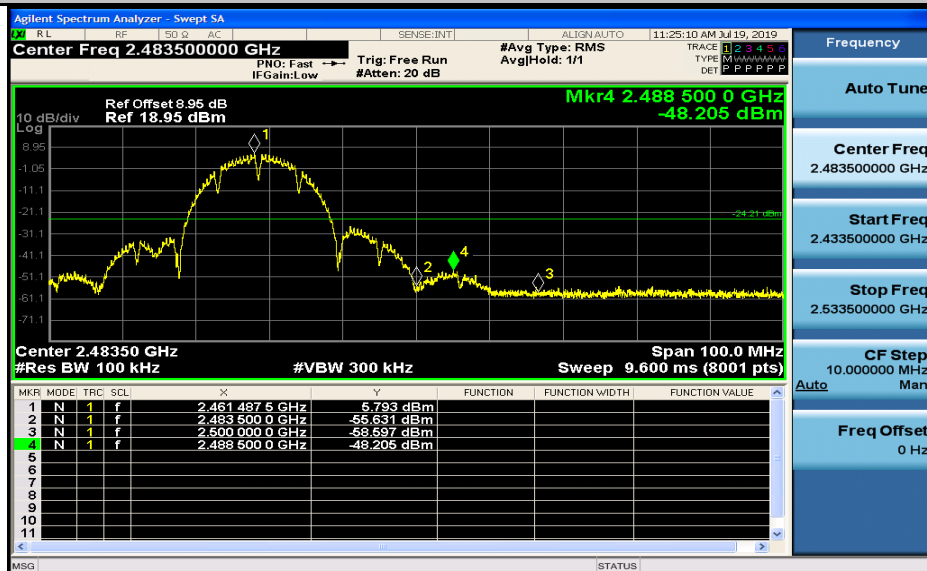
Band-edge for RF Conducted Emissions_11G_2412_Ant2
