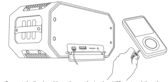
Connect the line in cable to the speaker's micro USB port and the other end to the audio source. Turn the speaker on and then press and hold the V -button for 2 seconds to enter line in mode. Please note only the volume controls work when connected via line in, you cannot skip or pause tracks.
