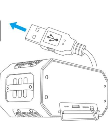
To charge your speaker connect the USB power cable to the micro USB port on the speaker and connect the other end to your computer's USB port. Whilst charging the LED indicator will turn red. When fully charged the red LED indicator will turn off. It will take up to 4 hours to fully charge the speaker.
