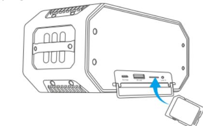
Use your computer to transfer music files to your microSD card. The speaker recognises MP3 audio files. Turn the speaker on and insert your microSD card into the microSD slot. The speaker will change to microSD mode and the music will start to play automatically.
