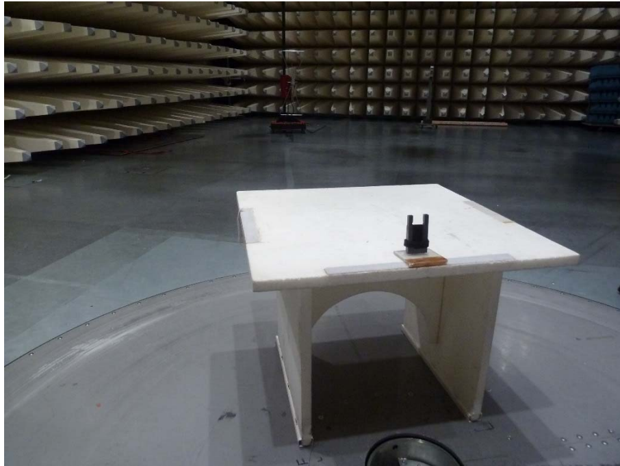
Photo 7: EUT at the semi-anechoic chamber
