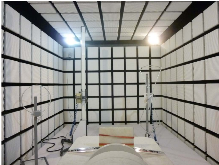
Photo 3: EUT at the anechoic chamber
