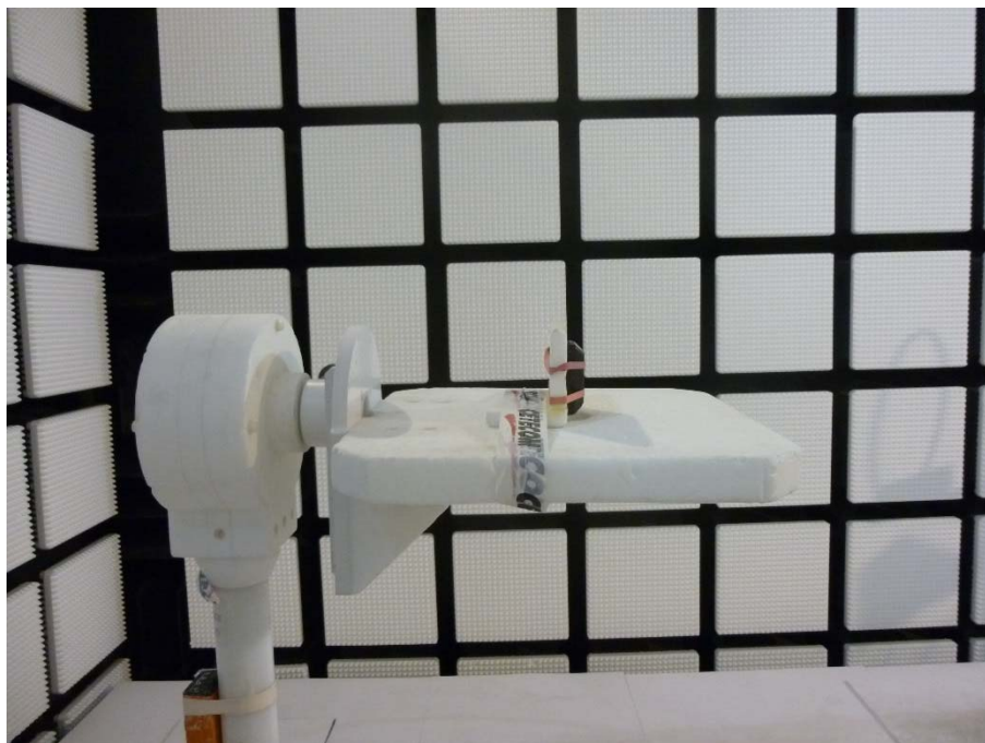
Photo 2: EUT at the anechoic chamber
