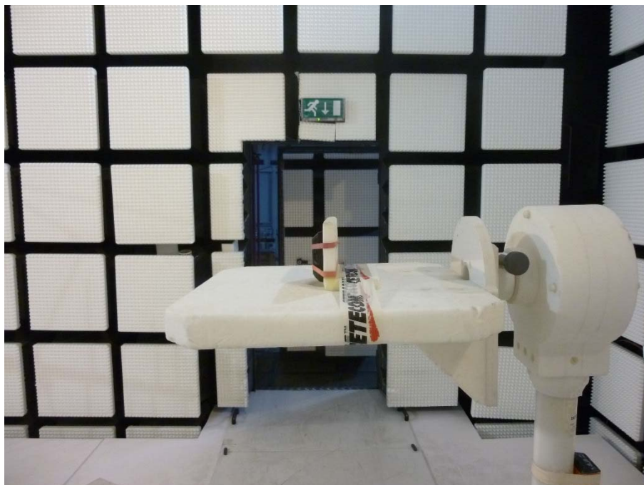
Photo 4: EUT at the anechoic chamber
