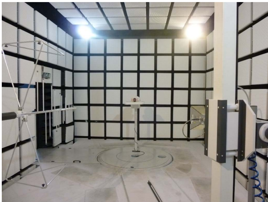
Photo 6: EUT at the anechoic chamber
