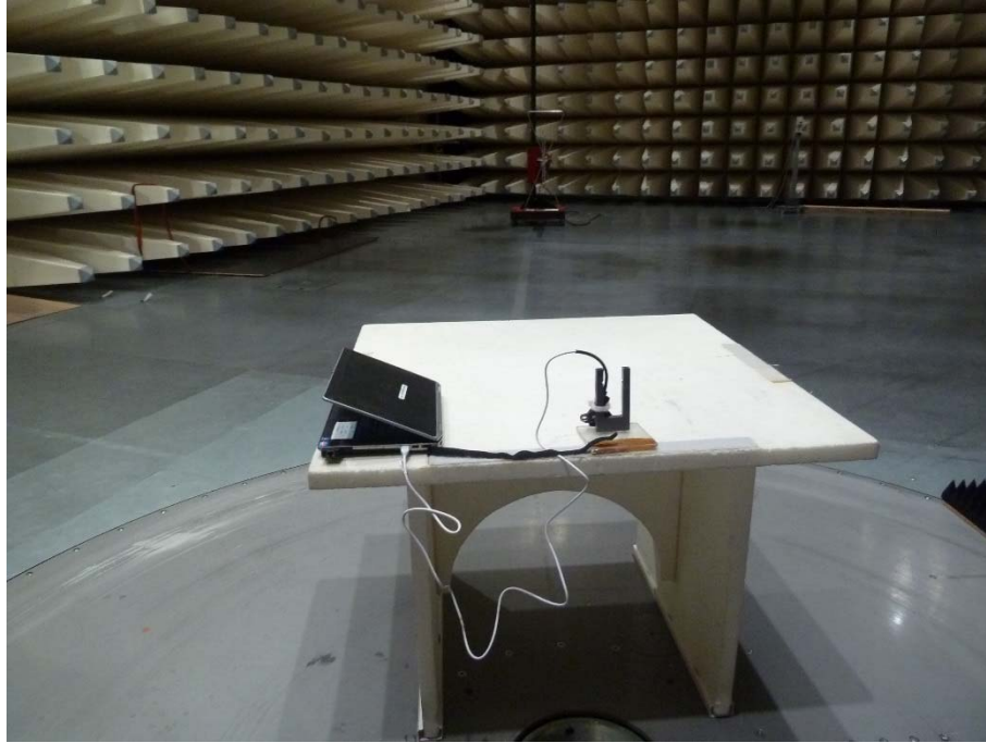
Photo 7: EUT at the semi-anechoic chamber
