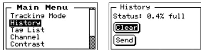
If connected to the RangeWATCH mobile app over Bluetooth, the history (including IDs, and transmission dates and times) can be sent to your tablet or smart phone by highlighting "Send" and pressing OK. Exit the menu by pressing MENU twice.
