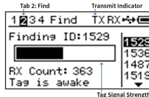
When in Find Mode, the RangeTRACKER can only wake up and find tags that are in its tag list. To change which ID in the tag list is being tracked by using UP ARROW and DOWN ARROW when in Find Mode. See 5.0 *Editing the Tag List* for more details about adding and removing tags from the list.
