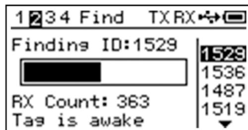
Change which ID in the list is being tracked by using UP ARROW and DOWN ARROW from the main windows, as shown above.
