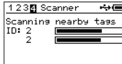
This mode is especially useful when the RangeTRACKER is paired with the RangeWATCH mobile app via Bluetooth. When the RangeTRACKER is in range of a mobile device (a tablet or a cell phone) running RangeWATCH mobile app, the app will automatically connect to the RangeTRACKER over Bluetooth. Tag reads in Scanner Mode are then used to track animal handling.
