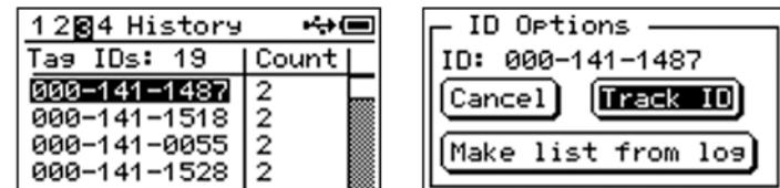
When you select Track ID, the specified ID will be added to the Tag List, and the RangeTRACKER will automatically transition to Find Mode to begin tracking the specified ID.
