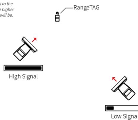
In Find Mode, the RangeTRACKER will also play a sound that matches the signal strength. Higher signal strength causes a higher-pitched tone to be played.
