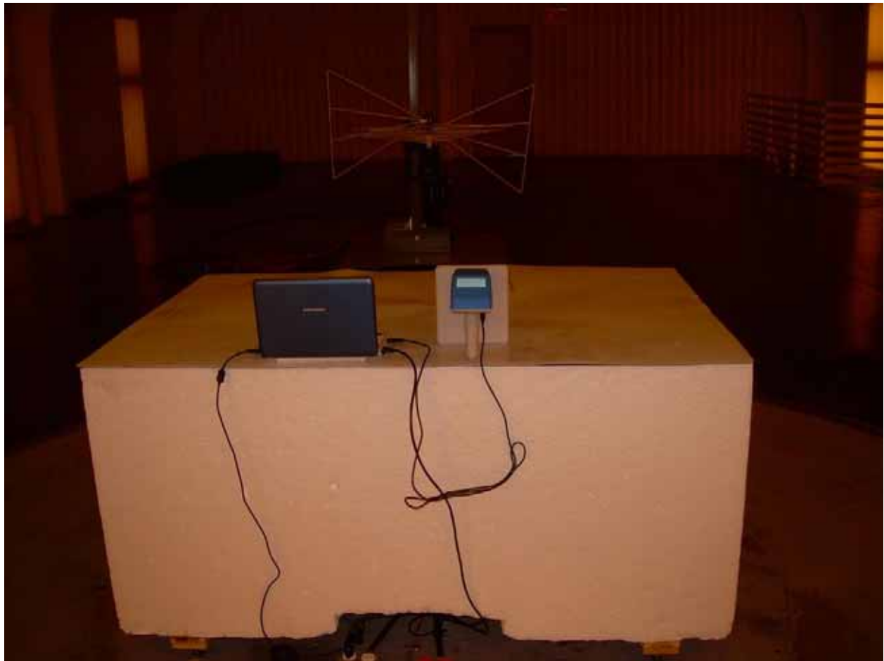
Photograph 2 – Back View Radiated Disturbance Worst Case Configuration – Connected to Computer Placed Vertical
