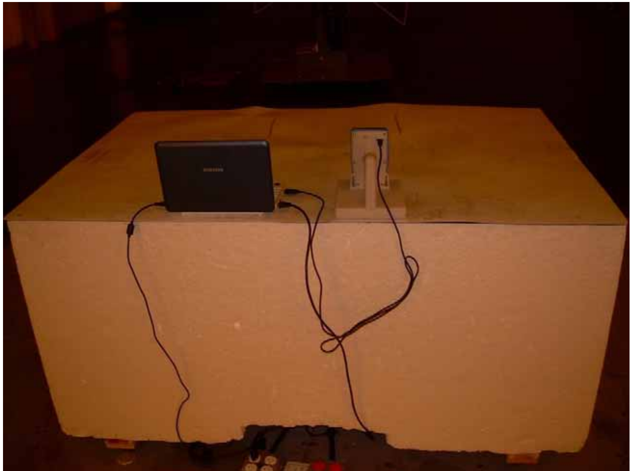
Photograph 6 – View Radiated Disturbance – Pointed Down Connected to Computer Configuration
