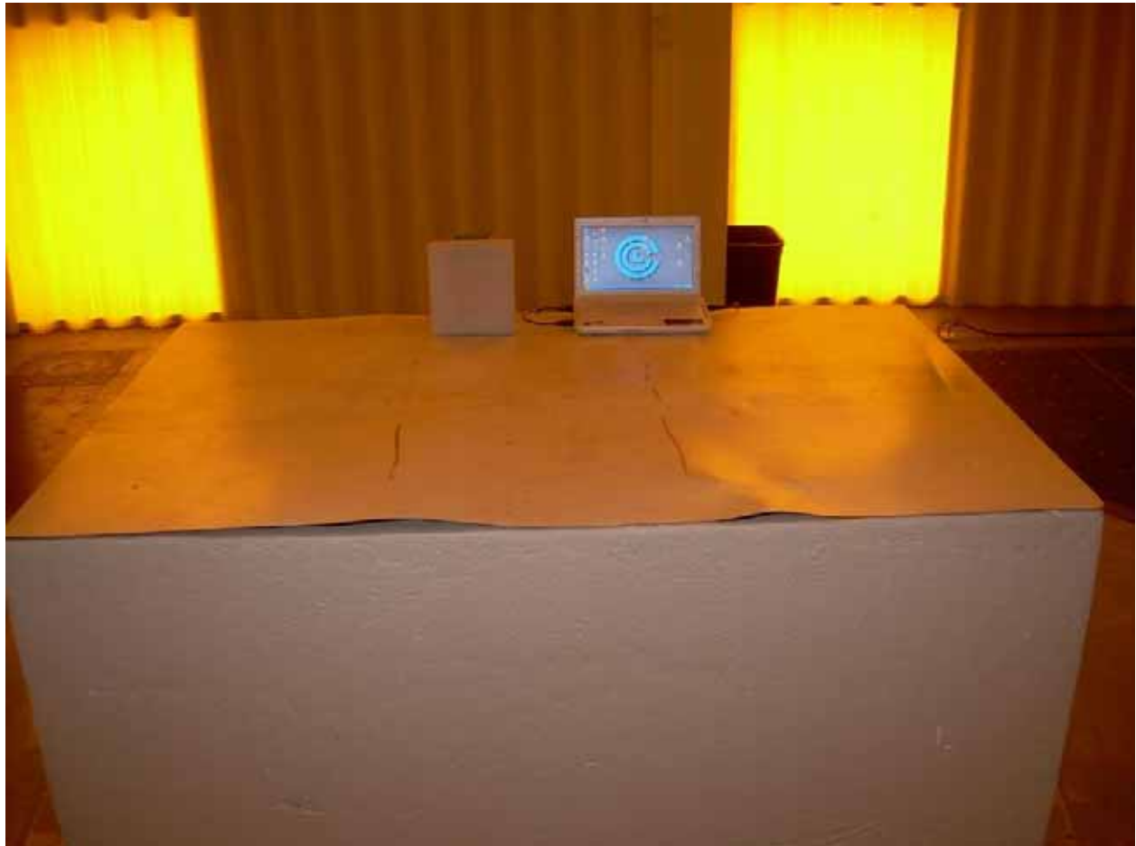
Photograph 1 – Front View Radiated Disturbance Worst Case Configuration – Connected to Computer Placed Vertical
