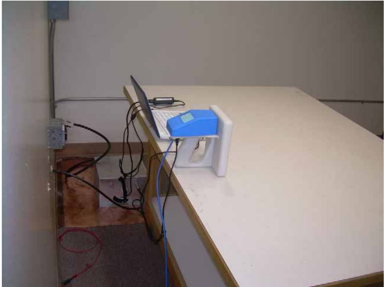
Photograph 9 – Back View Conducted Disturbance Worst Case Configuration
