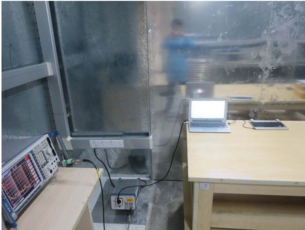
FCC RADIATED EMISSION TEST SETUP
