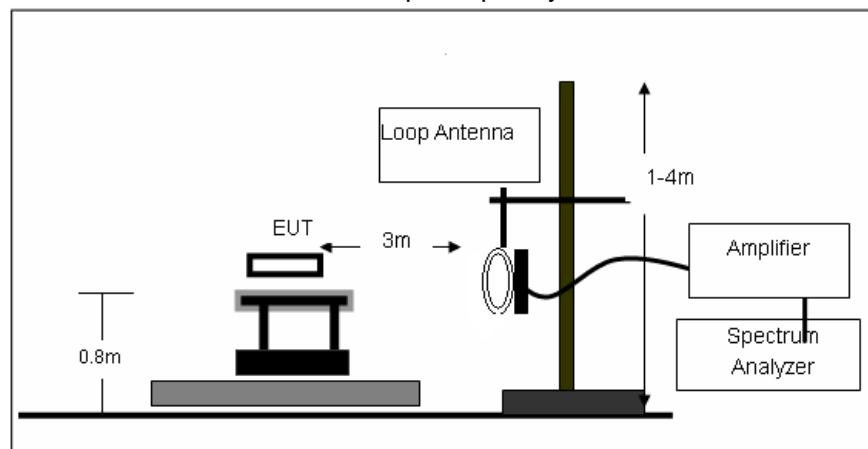
(2) Radiated Emission Test-Up Frequency 30MHz~1GHz
