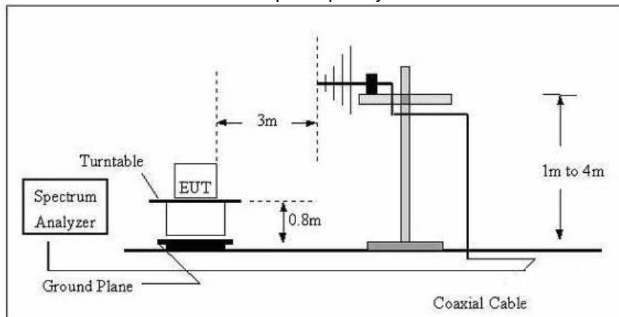
**(3) Radiated Emission Test-Up Frequency Above 1GHz**
