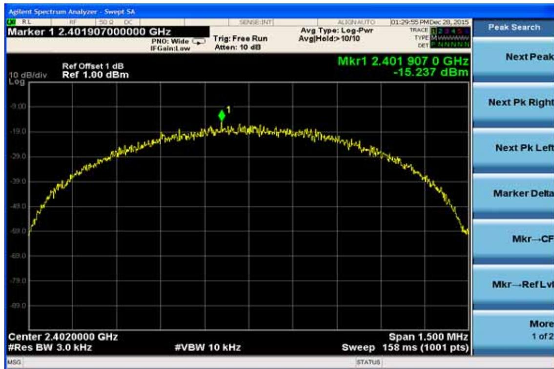
**Power Spectral Density Test Plot (CH-Mid)**
