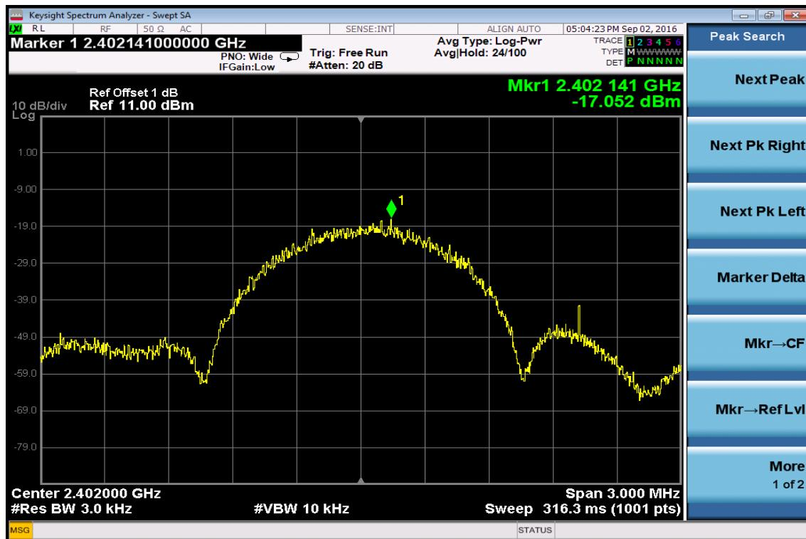
**Power Spectral Density Test Plot (CH-Mid)**
