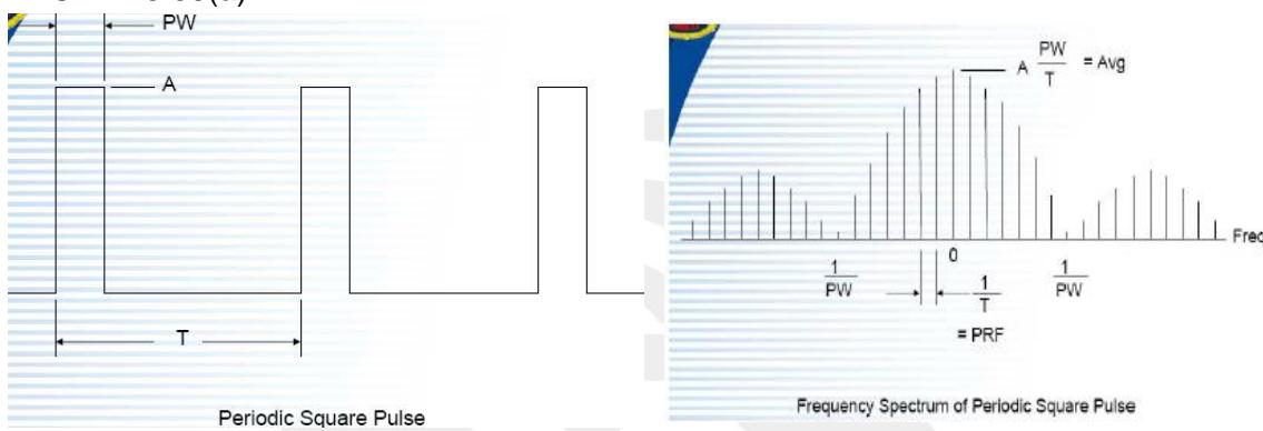
If using spectrum analyzer to measure pulse signal , it have to make sure the RBW use is at least  $2/PW$ .
