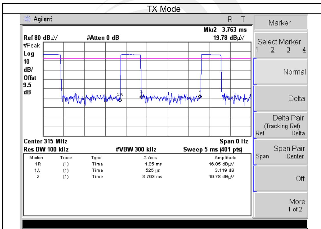
Refer to the plot (As Below), We find a manually operated transmitter shall employ a switch that will automatically deactivate the transmitter immediately, within not more than 5 seconds of being released.
