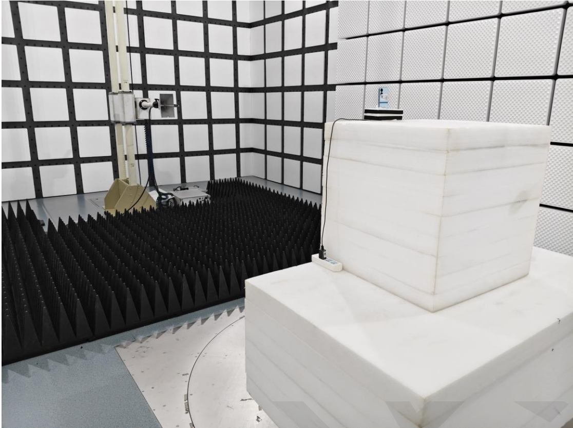
Radiated Spurious Emissions Test View (1GHz-18GHz)
