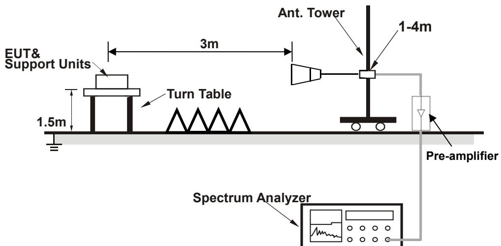
**For radiated test above 18GHz**
