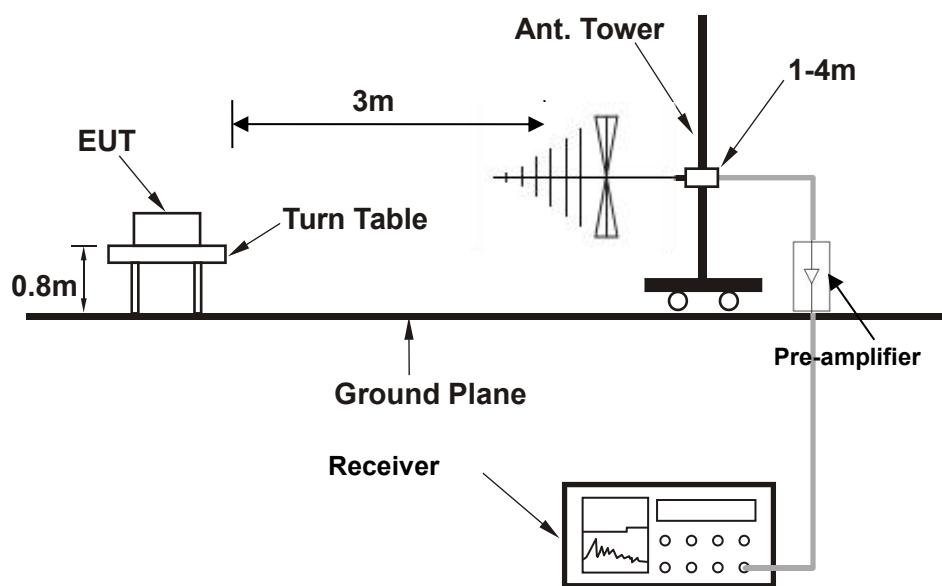
**For radiated test from 1GHz to 18GHz**
