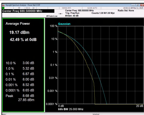
n71 SCS=15kHz DFT_256QAM BW=20MHz Channel=136100 RB=100@0
