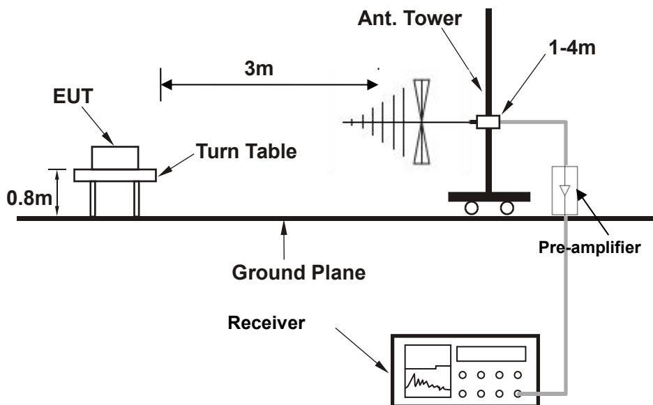
**For radiated test from 1GHz to 18GHz**
