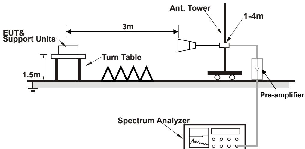
**For radiated test above 18GHz**
