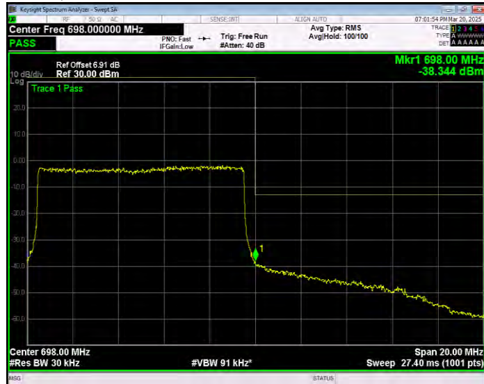
Band71 16QAM BW=10MHz Channel=133422 RB Size=1 Position=#Max Normal
