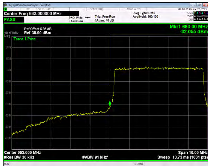
Band71 QPSK BW=5MHz Channel=133447 RB Size=1 Position=#Max Normal
