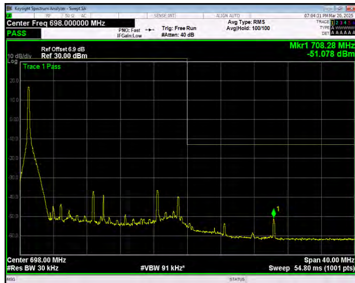
Band71 QPSK BW=20MHz Channel=133372 RB Size=1 Position=#Max Normal
