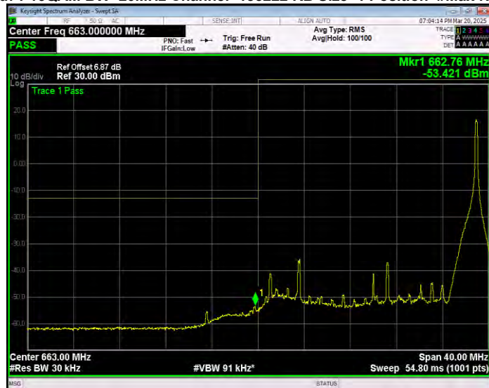
Band71 16QAM BW=20MHz Channel=133222 RB Size=100 Position=#0 Normal
