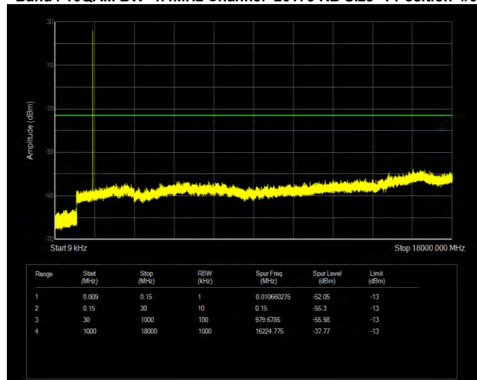
Band4 16QAM BW=10MHz Channel=20000 RB Size=1 Position=#0
