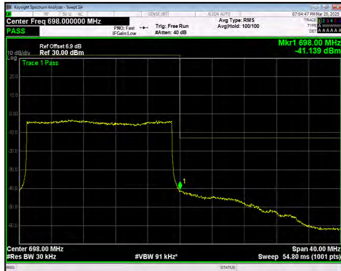
Band71 QPSK BW=5MHz Channel=133147 RB Size=1 Position=#Max Normal
