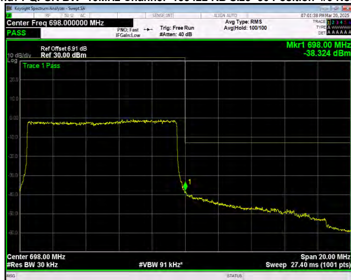
Band71 QPSK BW=15MHz Channel=133197 RB Size=1 Position=#0 Normal
