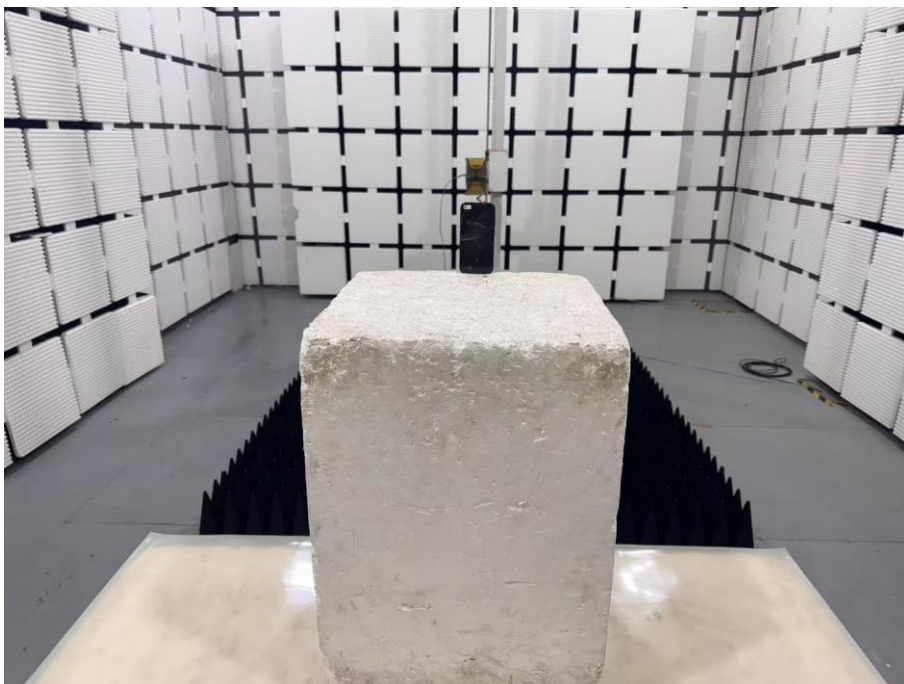
Set-up for Radiated Spurious Emission, Above 1GHz
