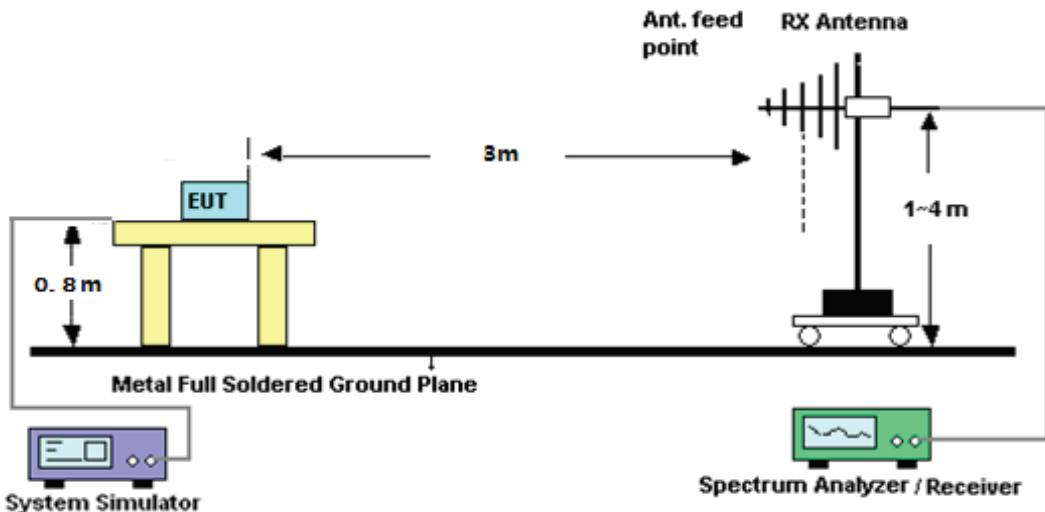
For radiated test from above 1GHz
