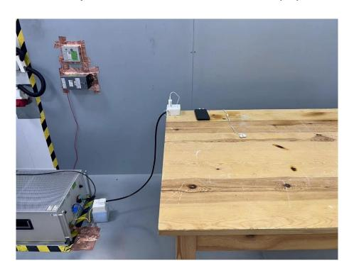
Set-up for Radiated Emission (RE), Below 1GHz
