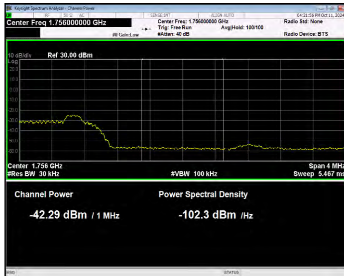
Band4 QPSK BW=5MHz Channel=20375 RB Size=1 Position=#0 Normal
