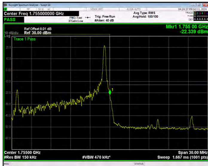
Band4 QPSK BW=15MHz Channel=20325 RB Size=75 Position=#0 Extended
