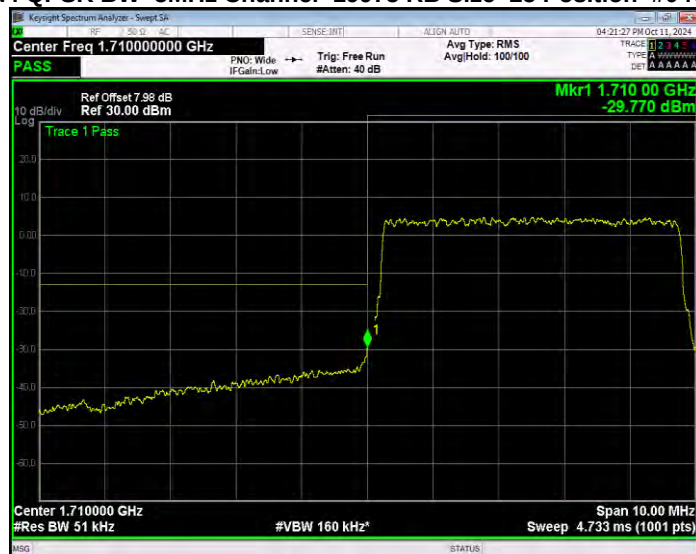
Band4 QPSK BW=5MHz Channel=20375 RB Size=1 Position=#0 Extended
