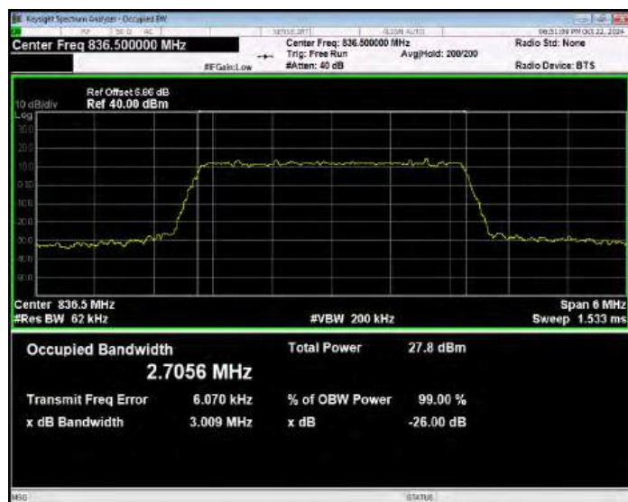
Band26(824-849) QPSK BW=3MHz Channel=27025 RB Size=15 Position=#0
