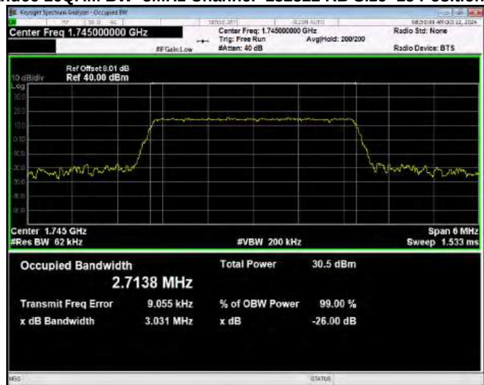
Band66 16QAM BW=3MHz Channel=132657 RB Size=15 Position=#0
