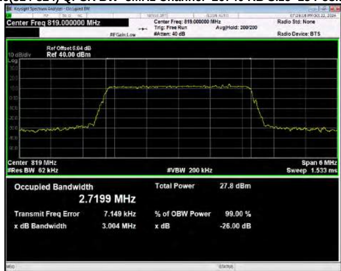
Band26(814-824) QPSK BW=3MHz Channel=26775 RB Size=15 Position=#0
