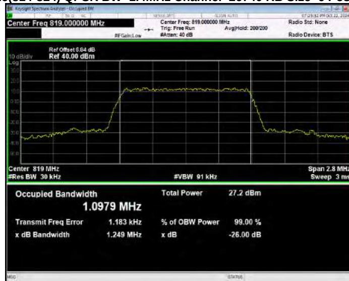
Band26(814-824) QPSK BW=1.4MHz Channel=26783 RB Size=6 Position=#0
