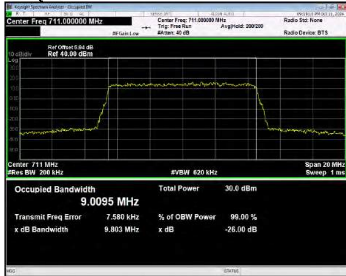
Band17 QPSK BW=5MHz Channel=23755 RB Size=25 Position=#0
