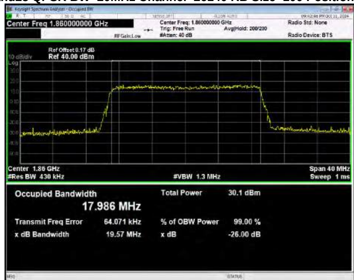
Band25 QPSK BW=20MHz Channel=26365 RB Size=100 Position=#0
