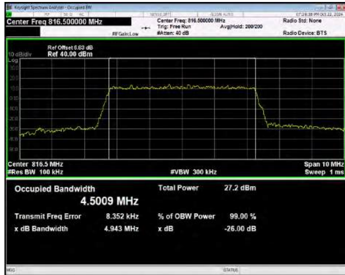
Band26(814-824) 16QAM BW=5MHz Channel=26740 RB Size=25 Position=#0
