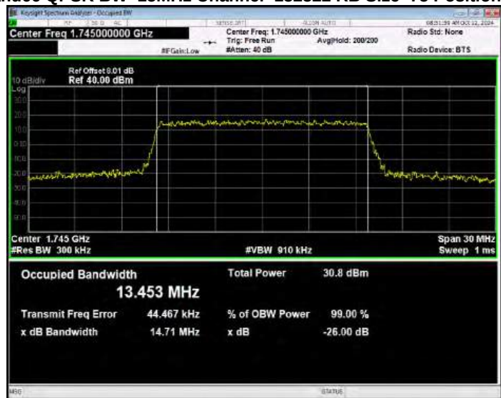
Band66 QPSK BW=15MHz Channel=132597 RB Size=75 Position=#0
