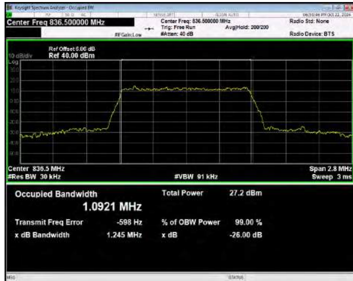
Band26(824-849) 16QAM BW=1.4MHz Channel=27033 RB Size=6 Position=#0
