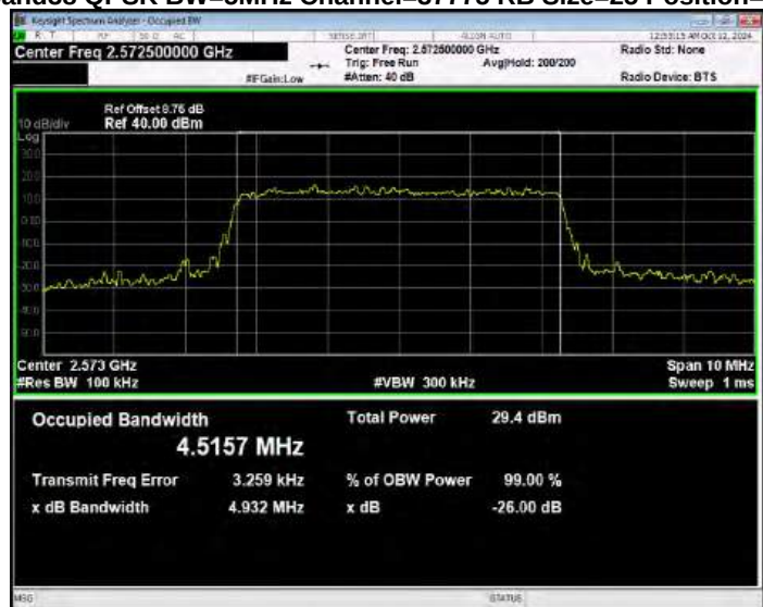
Band38 QPSK BW=5MHz Channel=38000 RB Size=25 Position=#0
