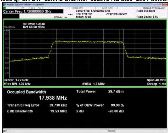
Band66 QPSK BW=20MHz Channel=132322 RB Size=100 Position=#0
