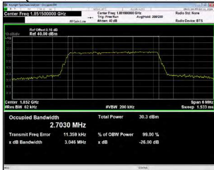
Band25 QPSK BW=3MHz Channel=26365 RB Size=15 Position=#0
