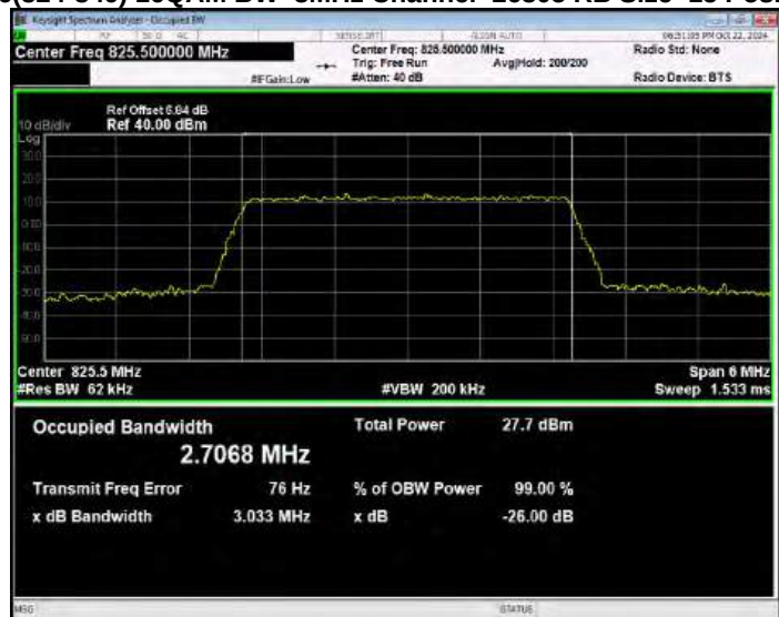
Band26(824-849) 16QAM BW=3MHz Channel=26915 RB Size=15 Position=#0
