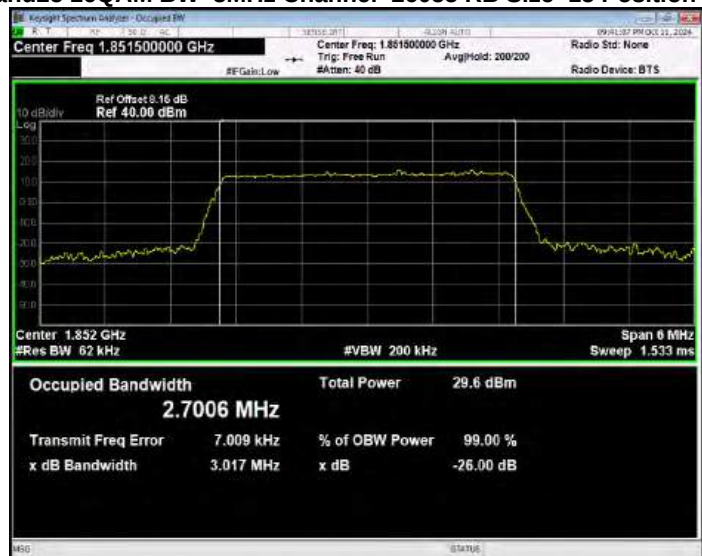
Band25 16QAM BW=3MHz Channel=26365 RB Size=15 Position=#0
