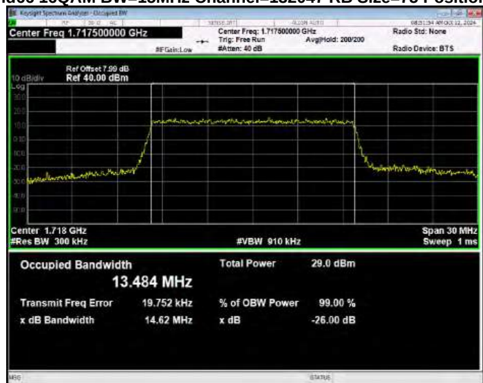
Band66 16QAM BW=15MHz Channel=132322 RB Size=75 Position=#0
