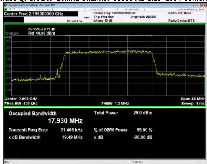
Band38 QPSK BW=20MHz Channel=38150 RB Size=100 Position=#0
