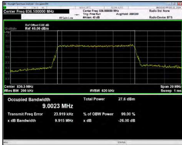
Band26(824-849) 16QAM BW=10MHz Channel=26990 RB Size=50 Position=#0
