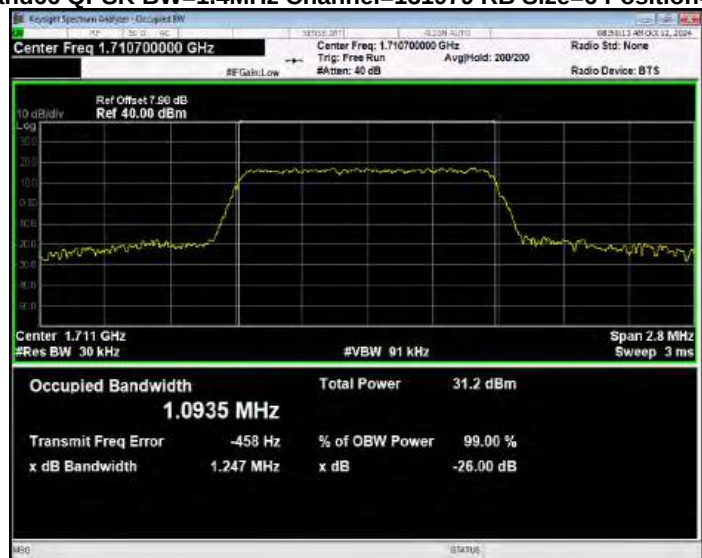
Band66 QPSK BW=1.4MHz Channel=132322 RB Size=6 Position=#0
