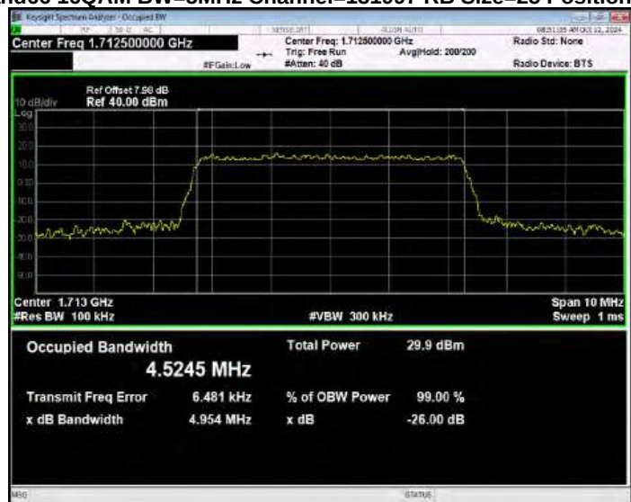
Band66 16QAM BW=5MHz Channel=132322 RB Size=25 Position=#0
