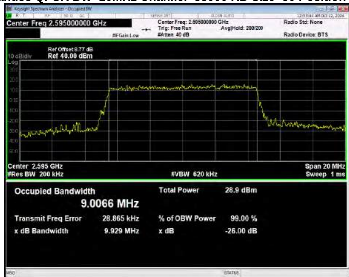
Band38 QPSK BW=10MHz Channel=38200 RB Size=50 Position=#0
