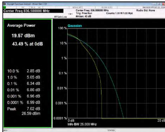
Band26(824-849) 16QAM BW=10MHz Channel=26990 RB Size=1 Position=#0
