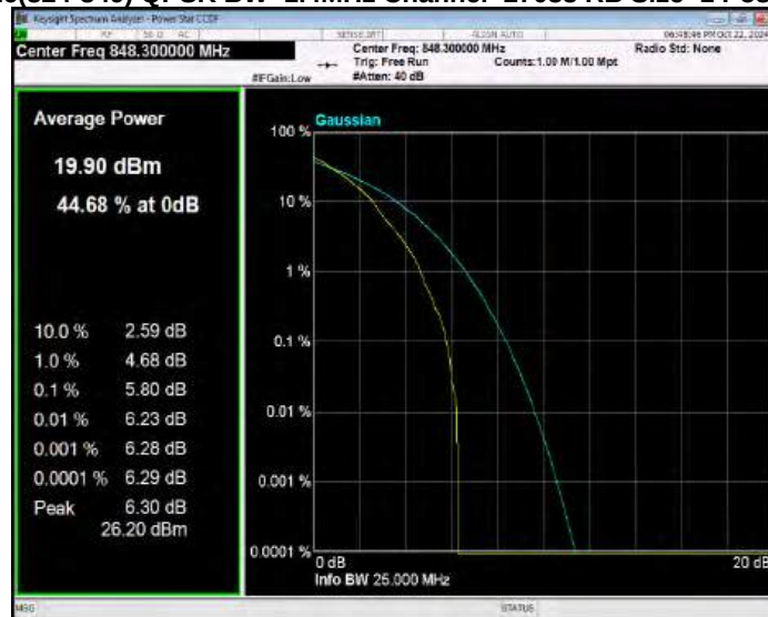
Band26(824-849) QPSK BW=10MHz Channel=26840 RB Size=1 Position=#0
