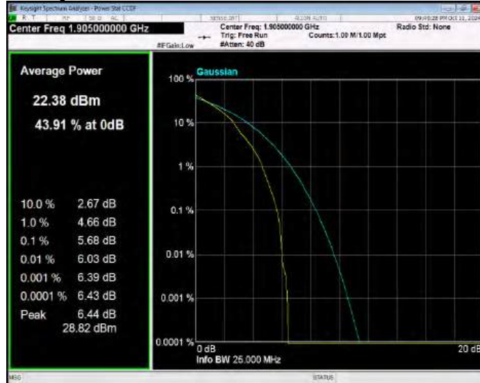
Band25 QPSK BW=3MHz Channel=26055 RB Size=1 Position=#0
