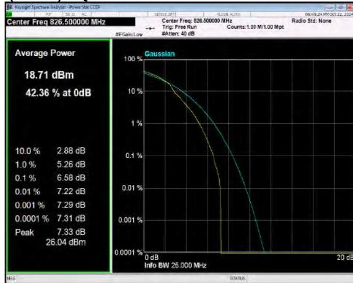
Band26(824-849) 16QAM BW=5MHz Channel=26915 RB Size=1 Position=#0
