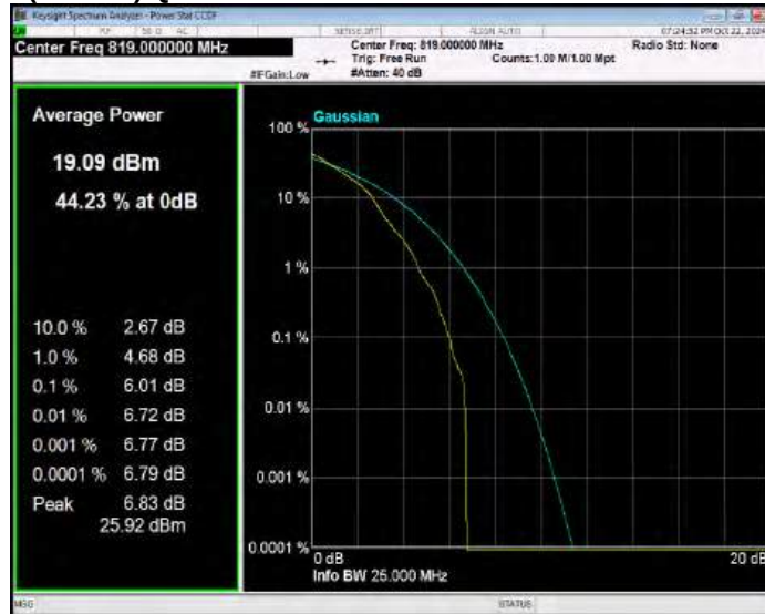
Band26(814-824) QPSK BW=3MHz Channel=26775 RB Size=1 Position=#0
