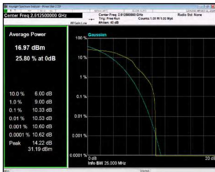
Band38 16QAM BW=20MHz Channel=37850 RB Size=1 Position=#0
