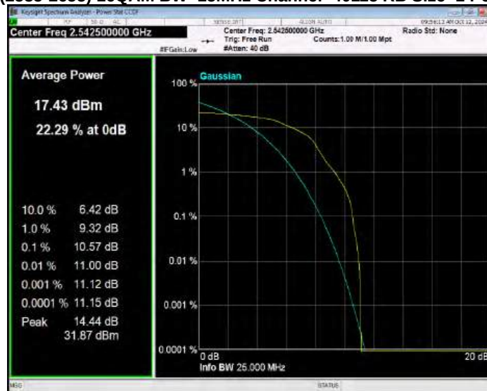
Band41(2535-2655) 16QAM BW=15MHz Channel=40640 RB Size=1 Position=#0
