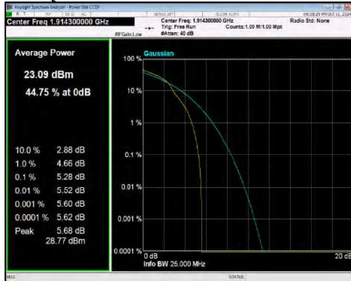
Band25 16QAM BW=10MHz Channel=26090 RB Size=1 Position=#0
