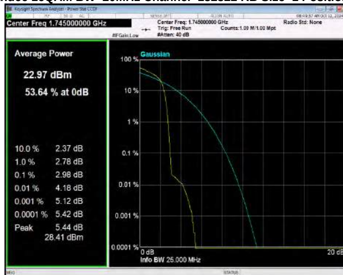
Band66 16QAM BW=20MHz Channel=132572 RB Size=1 Position=#0
