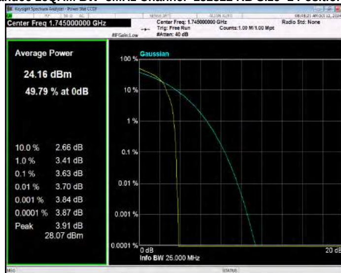
Band66 16QAM BW=3MHz Channel=132657 RB Size=1 Position=#0
