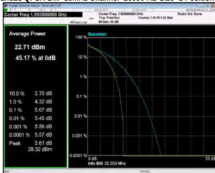
Band25 QPSK BW=10MHz Channel=26365 RB Size=1 Position=#0
