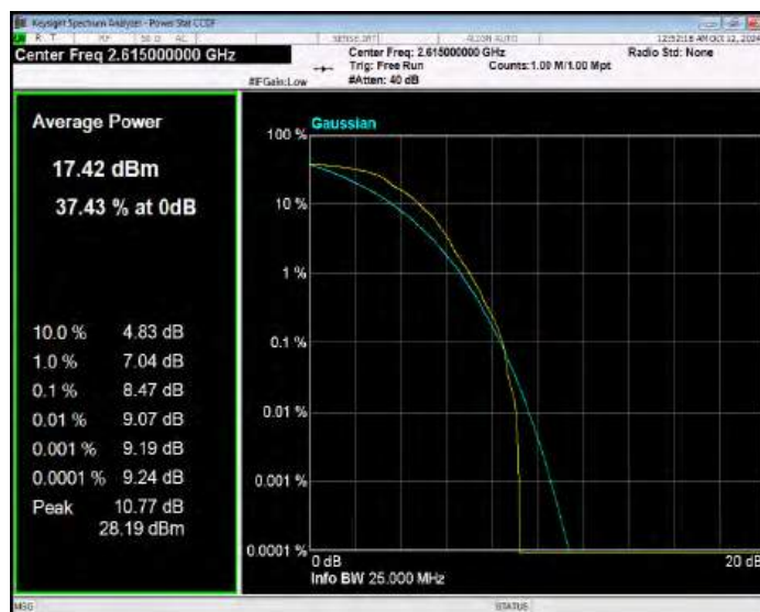
Band38 QPSK BW=15MHz Channel=37825 RB Size=1 Position=#0
