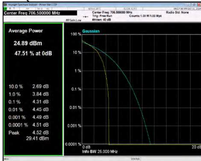
Band17 QPSK BW=5MHz Channel=23790 RB Size=1 Position=#0
