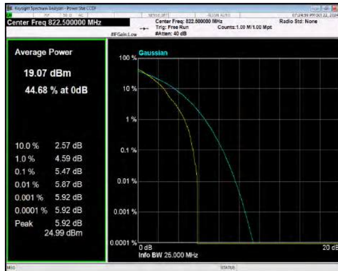
Band26(814-824) QPSK BW=5MHz Channel=26715 RB Size=1 Position=#0
