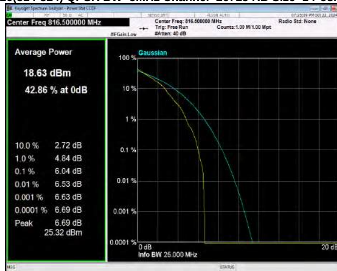
Band26(814-824) QPSK BW=5MHz Channel=26740 RB Size=1 Position=#0
