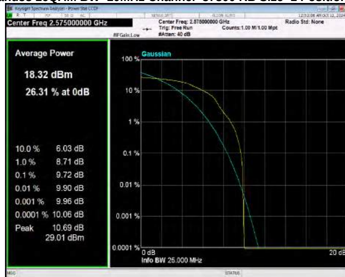
Band38 16QAM BW=10MHz Channel=38000 RB Size=1 Position=#0
