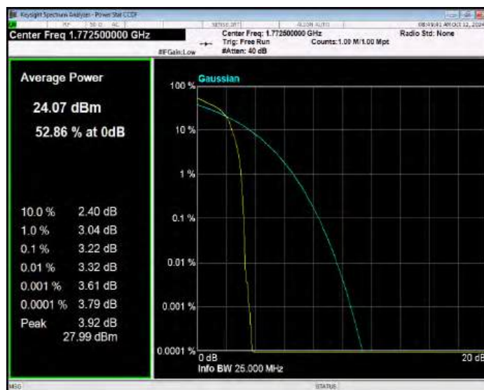
Band66 16QAM BW=20MHz Channel=132072 RB Size=1 Position=#0
