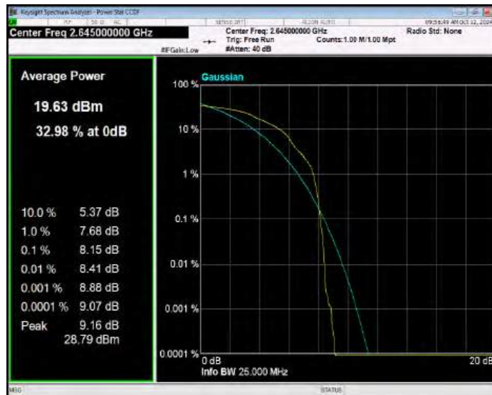
Band41(2535-2655) 16QAM BW=5MHz Channel=40065 RB Size=1 Position=#0
