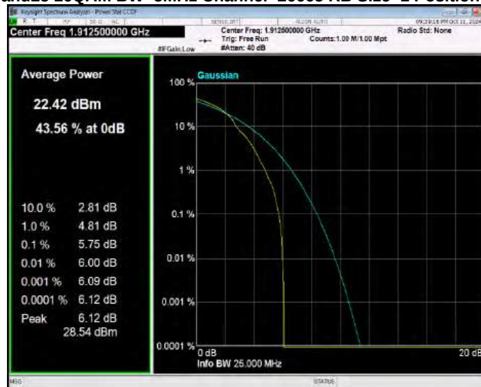
Band25 QPSK BW=1.4MHz Channel=26047 RB Size=1 Position=#0
