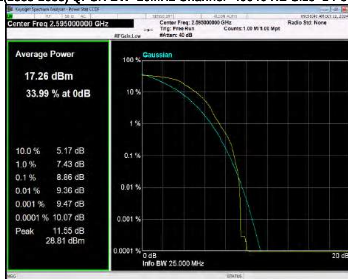
Band41(2535-2655) QPSK BW=20MHz Channel=41140 RB Size=1 Position=#0
