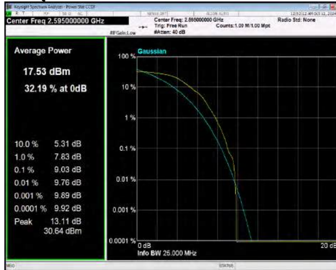
Band38 QPSK BW=10MHz Channel=38200 RB Size=1 Position=#0
