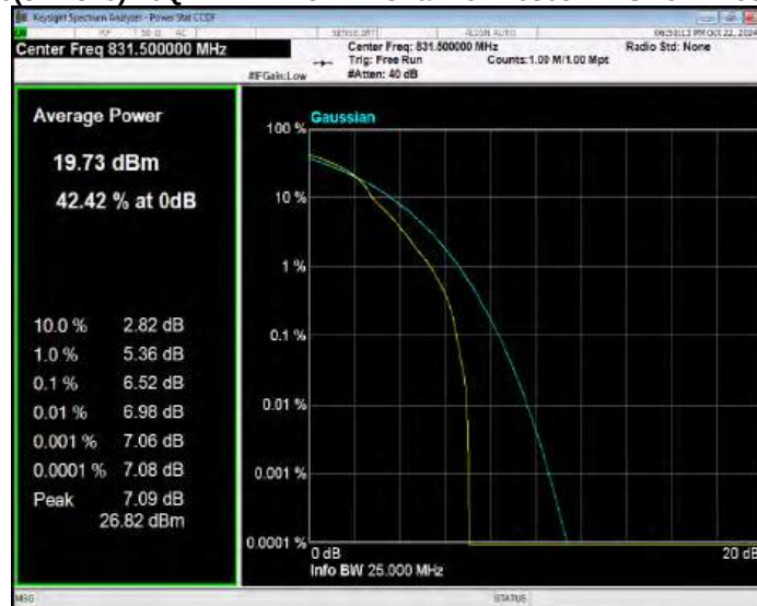
Band26(824-849) 16QAM BW=15MHz Channel=26915 RB Size=1 Position=#0
