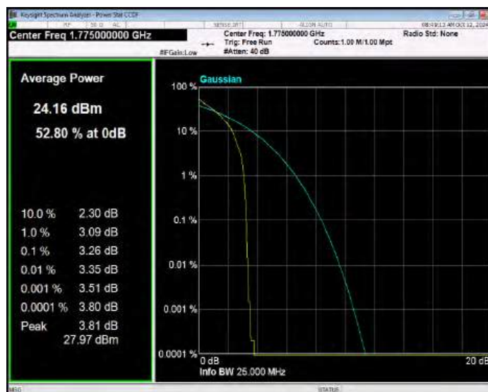
Band66 QPSK BW=15MHz Channel=132047 RB Size=1 Position=#0
