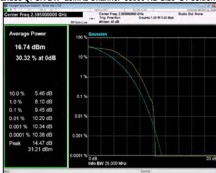
Band38 QPSK BW=15MHz Channel=38175 RB Size=1 Position=#0
