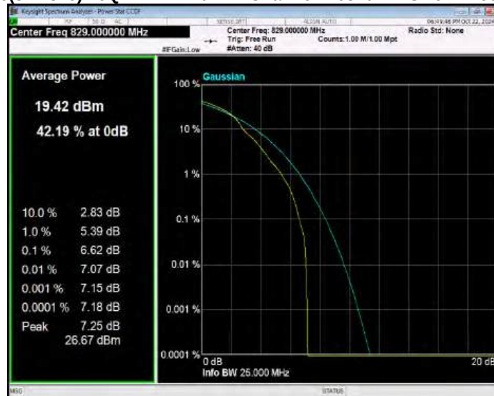
Band26(824-849) 16QAM BW=10MHz Channel=26915 RB Size=1 Position=#0
