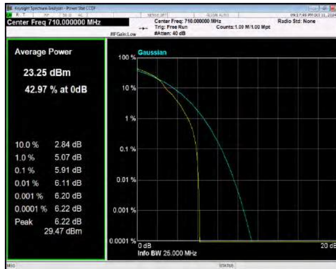
Band17 16QAM BW=5MHz Channel=23825 RB Size=1 Position=#0
