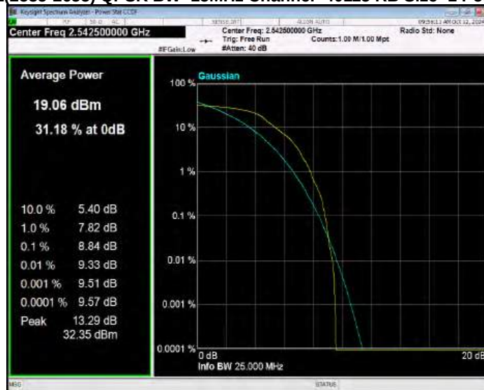
Band41(2535-2655) QPSK BW=15MHz Channel=40640 RB Size=1 Position=#0
