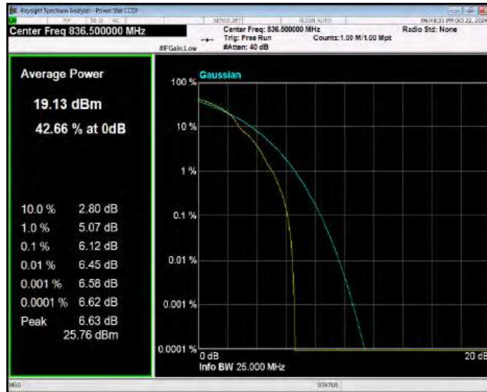
Band26(824-849) 16QAM BW=5MHz Channel=27015 RB Size=1 Position=#0
