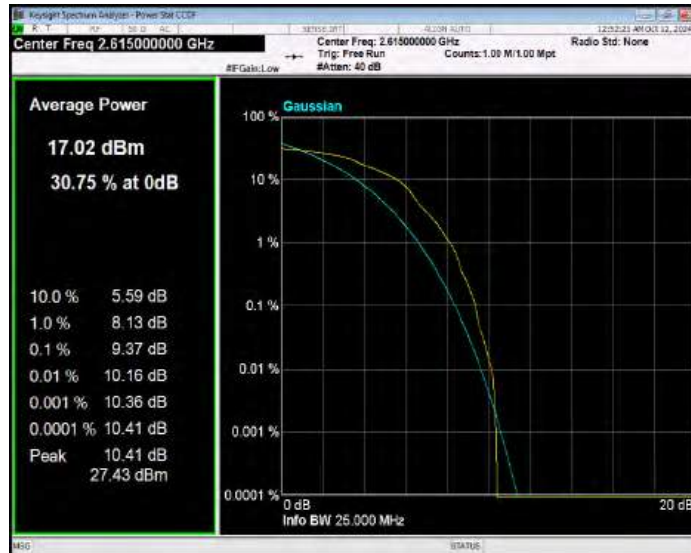
Band38 16QAM BW=15MHz Channel=37825 RB Size=1 Position=#0
