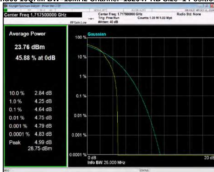
Band66 16QAM BW=15MHz Channel=132322 RB Size=1 Position=#0
