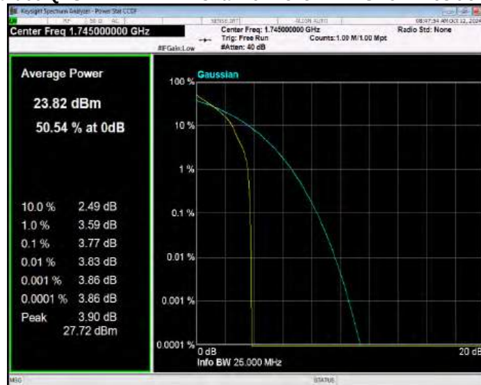
Band66 QPSK BW=1.4MHz Channel=132665 RB Size=1 Position=#0
