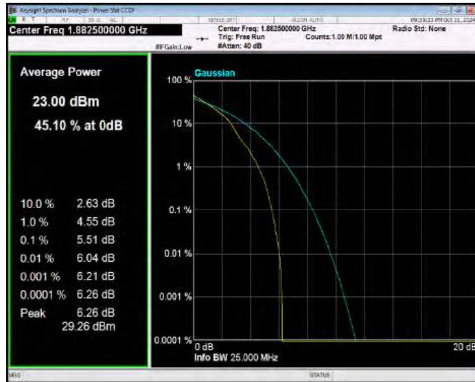
Band25 QPSK BW=10MHz Channel=26640 RB Size=1 Position=#0
