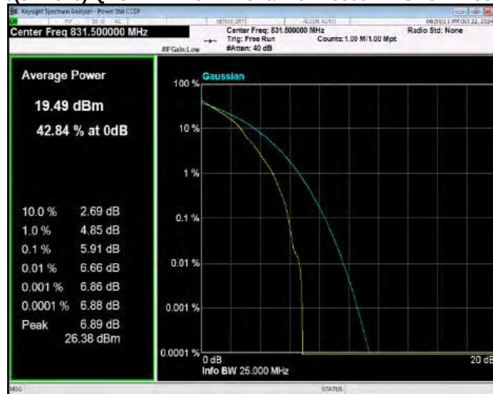
Band26(824-849) QPSK BW=15MHz Channel=26915 RB Size=1 Position=#0
