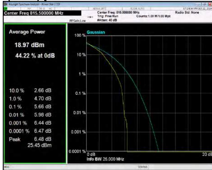
Band26(814-824) QPSK BW=3MHz Channel=26740 RB Size=1 Position=#0
