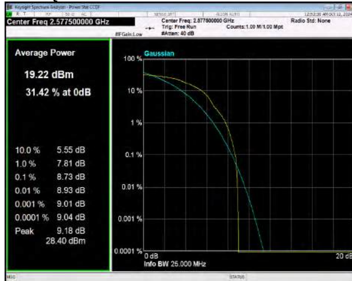
Band38 16QAM BW=15MHz Channel=38000 RB Size=1 Position=#0
