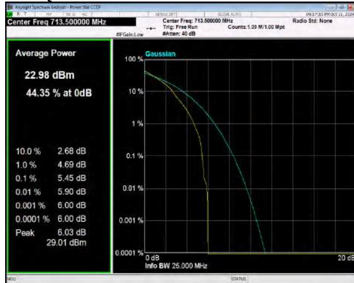
Band25 16QAM BW=1.4MHz Channel=26047 RB Size=1 Position=#0
