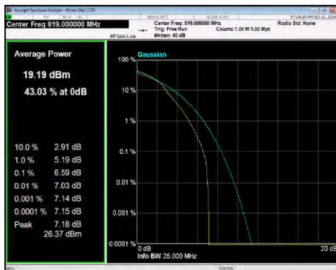
Band26(814-824) 16QAM BW=1.4MHz Channel=26783 RB Size=1 Position=#0
