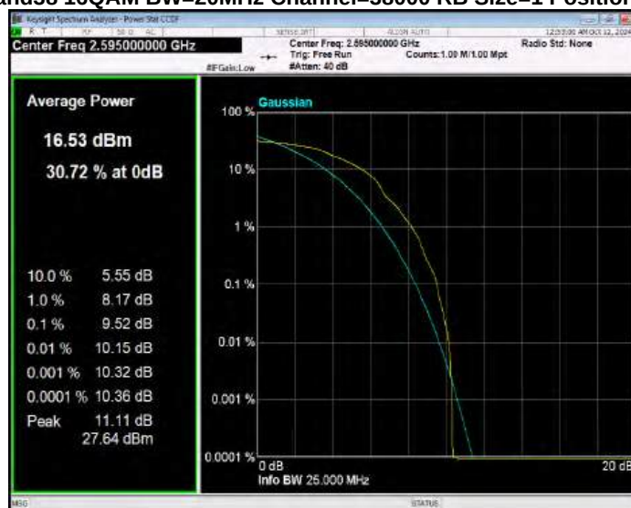
Band38 16QAM BW=20MHz Channel=38150 RB Size=1 Position=#0
