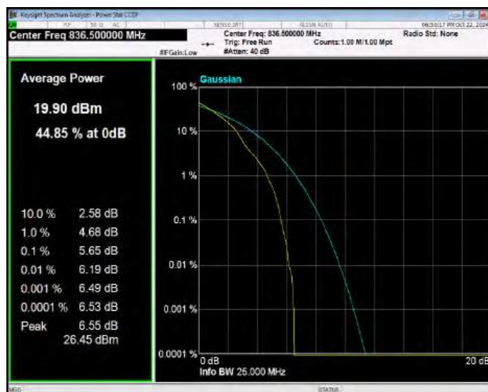
Band26(824-849) QPSK BW=15MHz Channel=26965 RB Size=1 Position=#0
