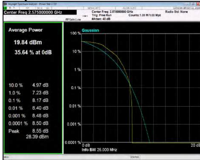
Band38 QPSK BW=10MHz Channel=38000 RB Size=1 Position=#0
