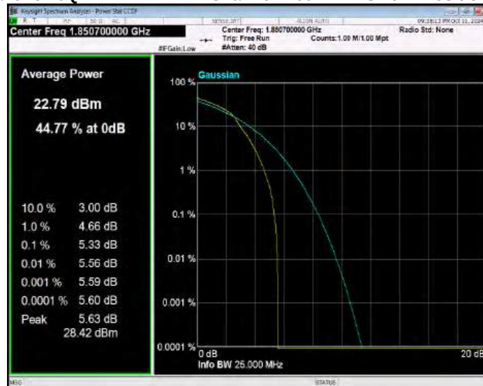
Band25 16QAM BW=1.4MHz Channel=26365 RB Size=1 Position=#0
