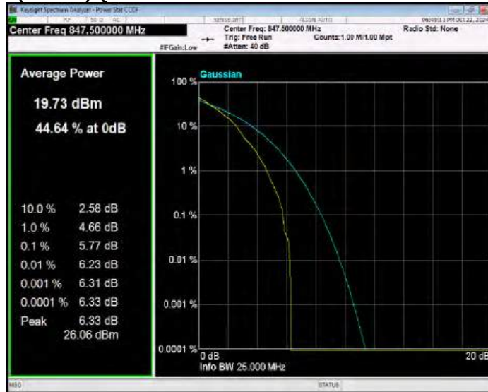
Band26(824-849) QPSK BW=5MHz Channel=26815 RB Size=1 Position=#0
