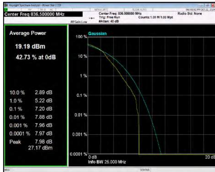
Band26(824-849) 16QAM BW=1.4MHz Channel=27033 RB Size=1 Position=#0
