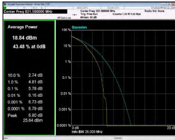
Band38 16QAM BW=10MHz Channel=37800 RB Size=1 Position=#0
