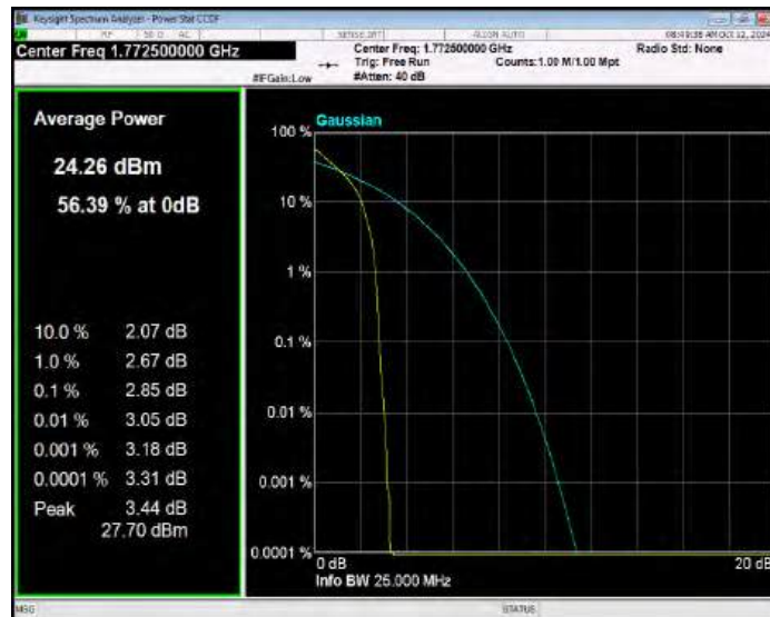
Band66 QPSK BW=20MHz Channel=132072 RB Size=1 Position=#0
