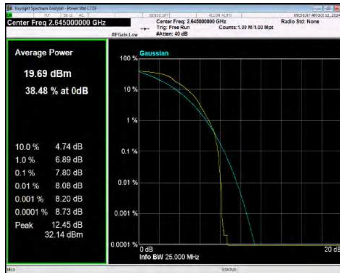
Band41(2535-2655) QPSK BW=5MHz Channel=40065 RB Size=1 Position=#0
