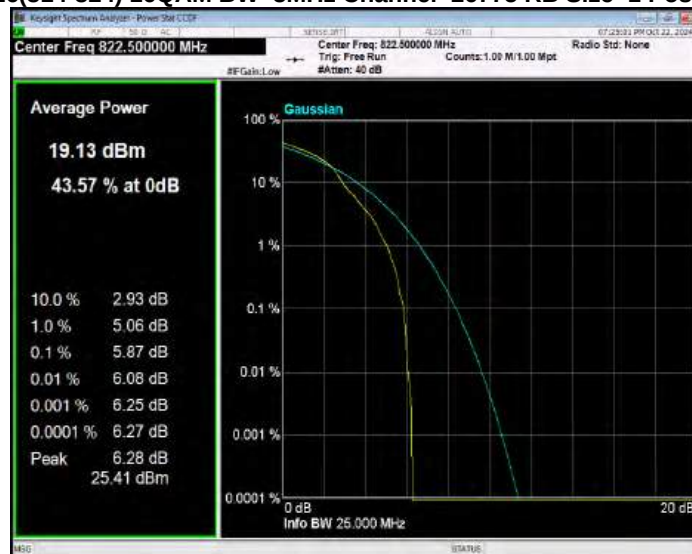
Band26(814-824) 16QAM BW=5MHz Channel=26715 RB Size=1 Position=#0
