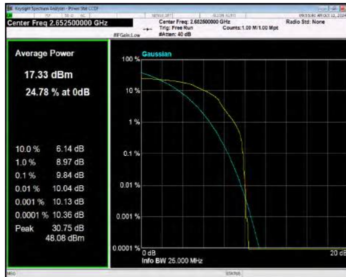
Band41(2535-2655) QPSK BW=10MHz Channel=40090 RB Size=1 Position=#0
