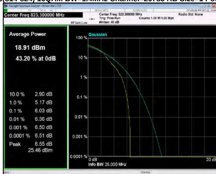
Band26(814-824) 16QAM BW=10MHz Channel=26740 RB Size=1 Position=#0
