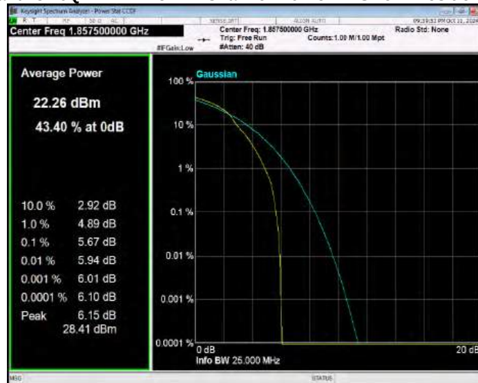
Band25 16QAM BW=15MHz Channel=26365 RB Size=1 Position=#0
