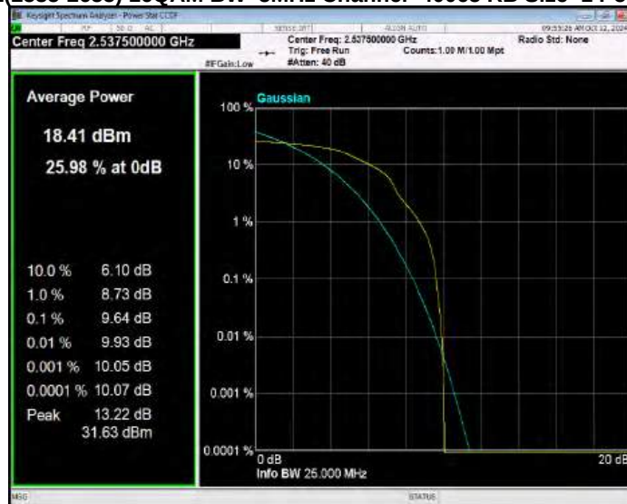
Band41(2535-2655) 16QAM BW=5MHz Channel=40640 RB Size=1 Position=#0
