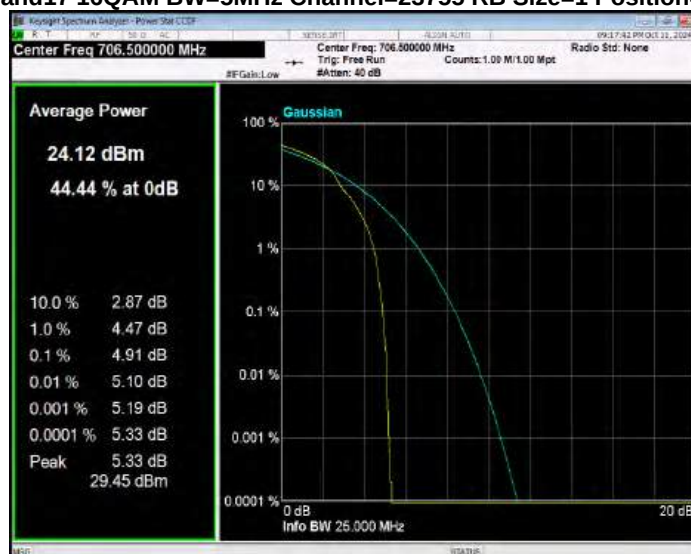
Band17 16QAM BW=5MHz Channel=23790 RB Size=1 Position=#0
