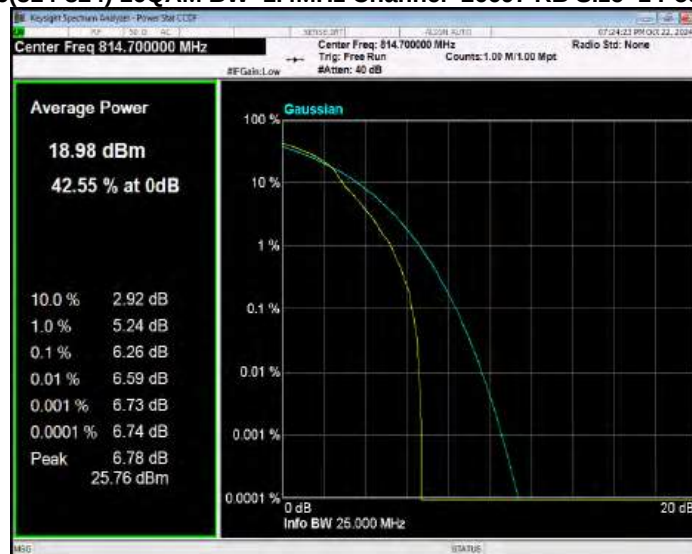
Band26(814-824) 16QAM BW=1.4MHz Channel=26740 RB Size=1 Position=#0
