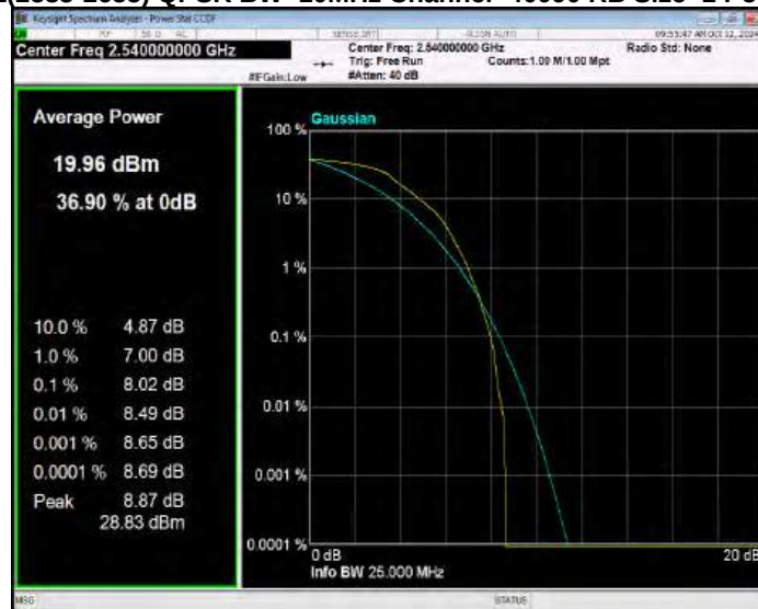
Band41(2535-2655) QPSK BW=10MHz Channel=40640 RB Size=1 Position=#0
