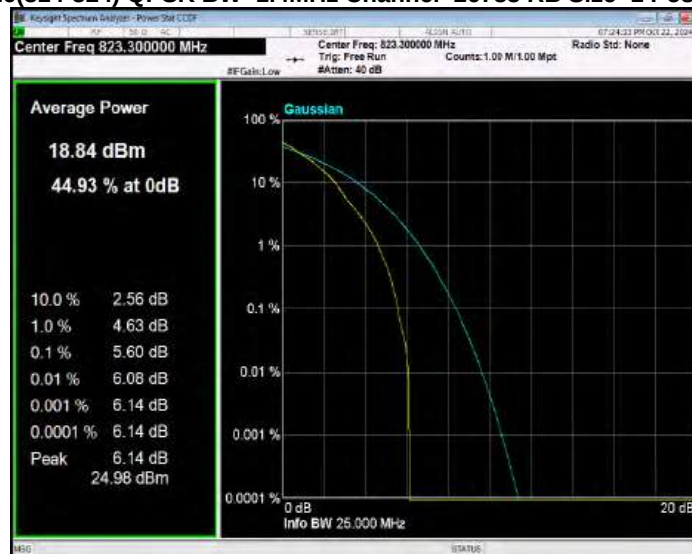
Band26(814-824) QPSK BW=10MHz Channel=26740 RB Size=1 Position=#0
