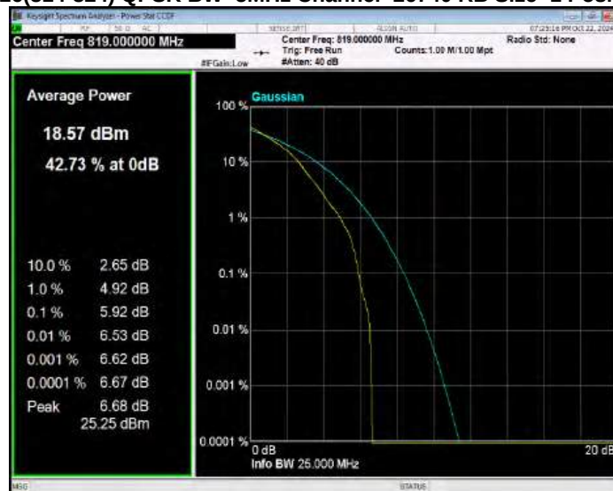
Band26(814-824) QPSK BW=5MHz Channel=26765 RB Size=1 Position=#0
