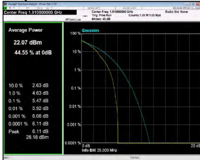
Band25 QPSK BW=15MHz Channel=26115 RB Size=1 Position=#0
