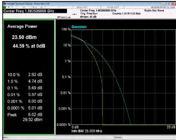
Band25 16QAM BW=3MHz Channel=26675 RB Size=1 Position=#0
