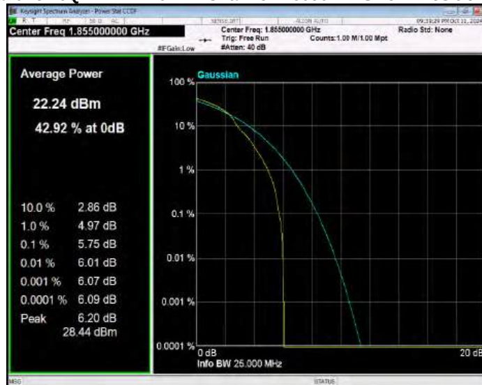
Band25 16QAM BW=10MHz Channel=26365 RB Size=1 Position=#0
