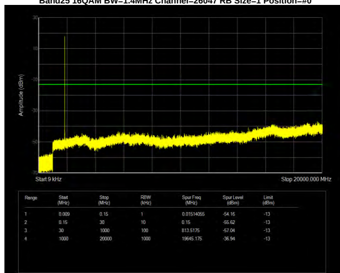
Band25 16QAM BW=1.4MHz Channel=26365 RB Size=1 Position=#0
