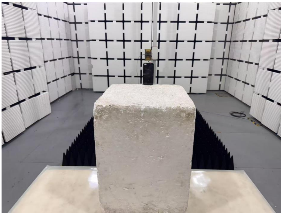
Set-up for Radiated Spurious Emission, Above 1GHz
