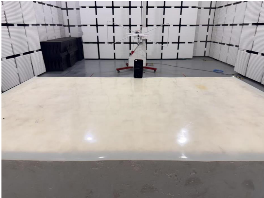
Set-up for Radiated Spurious Emission, Above 1GHz
