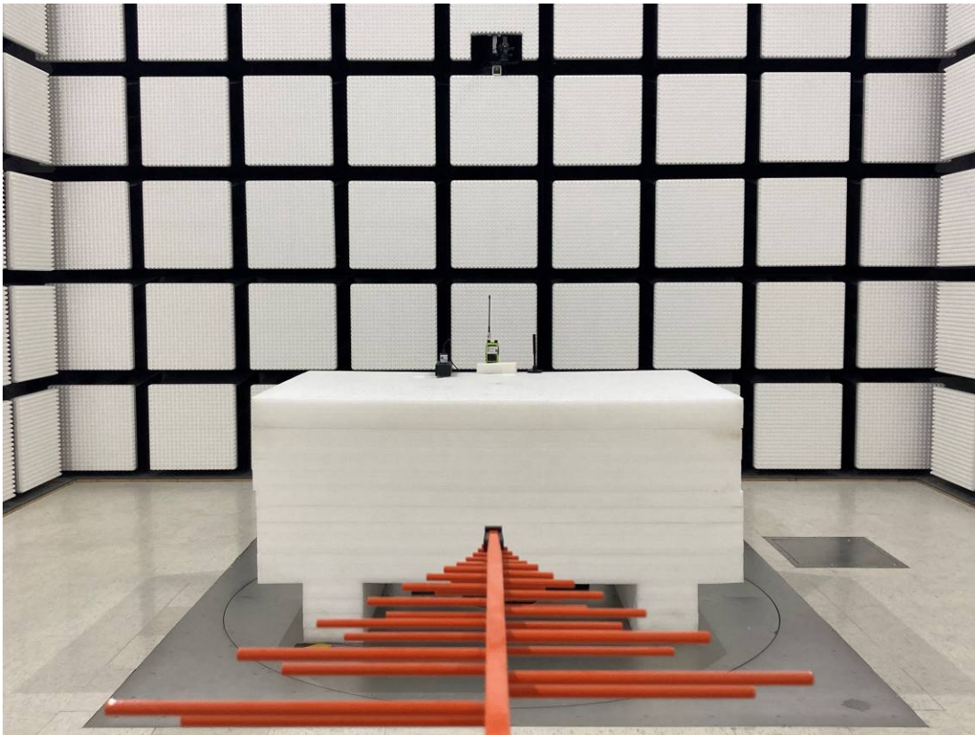
Radiated Emission Below 1GHz Rear View
