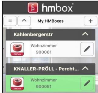
1. A **manual synchronisation** is **only** possible on site in the direct vicinity of the HMBox (~ 8m), Bluetooth connection must be active and sufficient network connection
