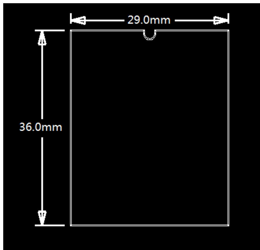
Thickness of module plate: 1.0mm
