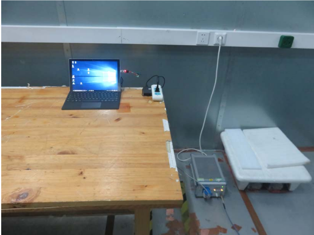
Picture 3 Conducted Emission Test Setup
