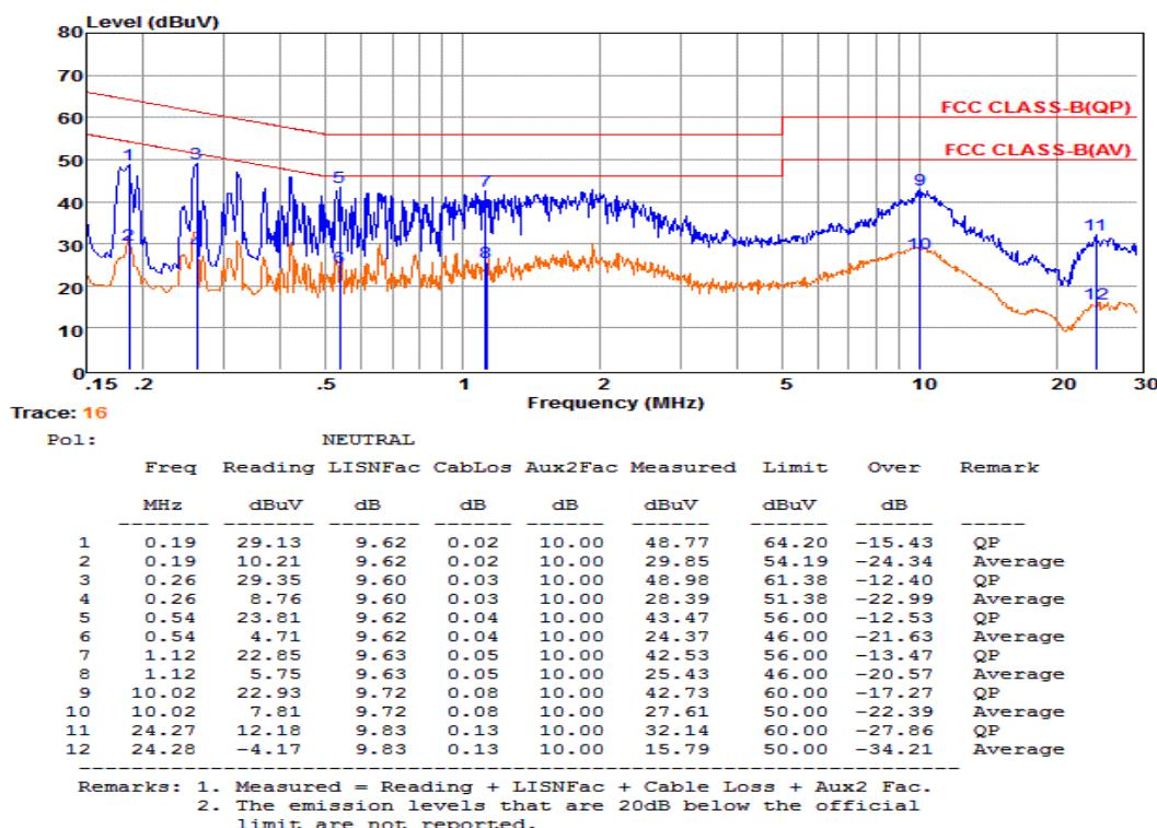
\*\*\*Note: Pre-scan all modes and recorded the worst case results in this report (IEEE 802.11ac VHT20 mode (High Channel, at Antenna Chain0)).
