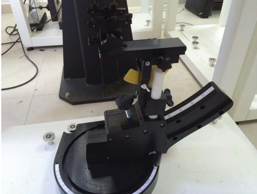
Device holder supplied by SPEAG
