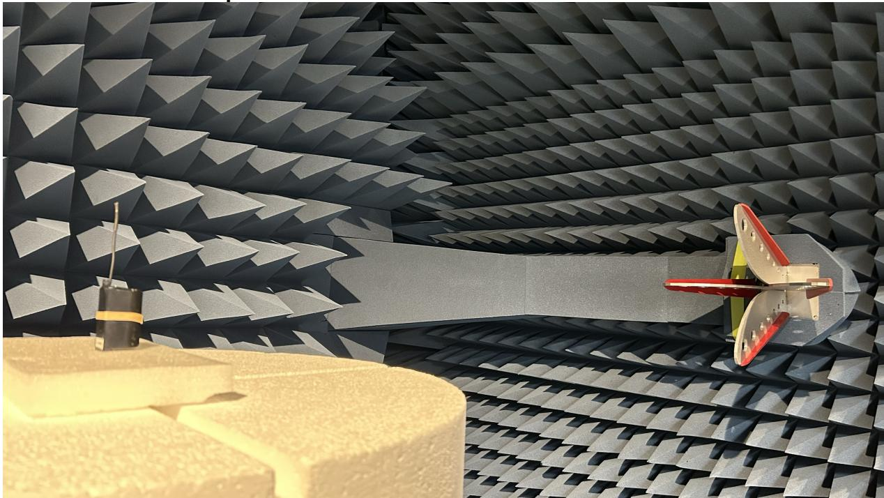
The EUT was placed on top of the Styrofoam mast in a holding fixture at the 0° position.
