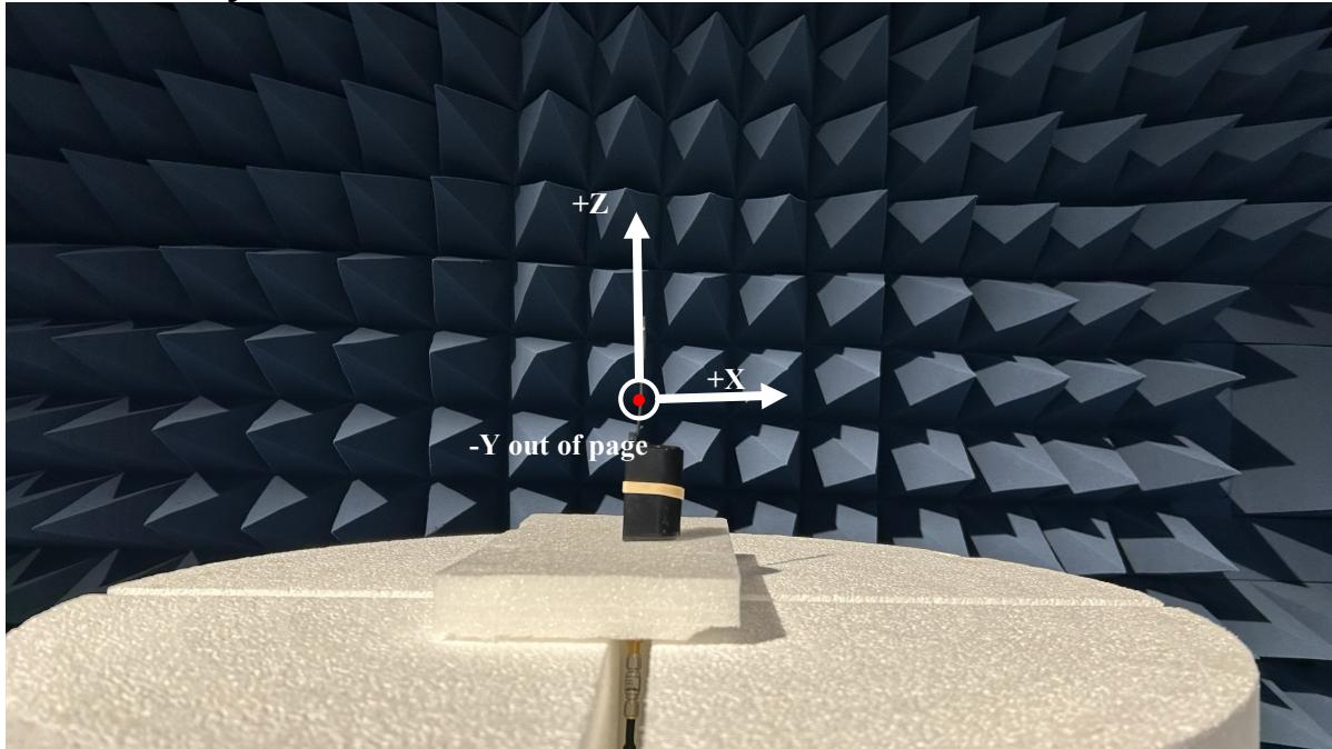
The coordinate system is centered on the DUT, with the -Y-axis pointing front side of the DUT, the +X-axis pointing right side of the DUT, and the +Z-axis pointing top side of the DUT.
